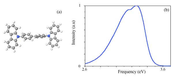
**Figure 2(a, b).** (color online) **(a)** A molecular structure of the CBP material (4,4'-Bis(*N*-carbazolyl)-1,1'-biphenyl). **(b)** An emission spectrum of 26 nm CBP on sapphire reference sample.
