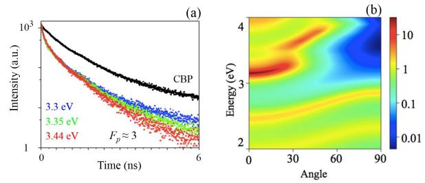
**Figure 3(a, b).** (color online) **(a)** Results of the TCSPC measurements. Black curve is decay curve of the 26 nm CBP reference sample at the frequency 3.35 eV. Blue, green and red curves are representing decay curves of Tamm plasmon structures at frequencies 3.3 eV, 3.35 eV, 3.44 eV, respectively. **(b)** The calculated distribution of the modal Purcell factor.
