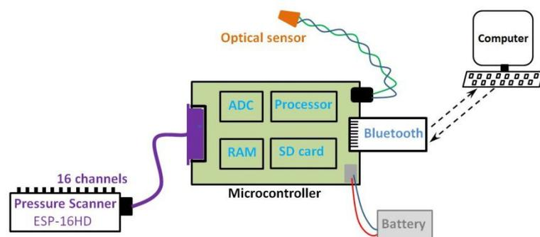
Figure 19 Schematic diagram of the microcontroller datalogger and other components<sup>5</sup>
