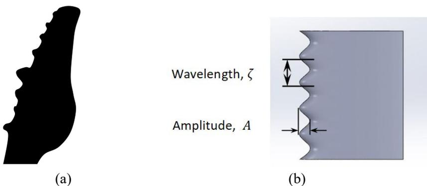
Figure 6 (a) Schematic drawing of the humpback whale flipper with large rounded tubercles along the leading edge and (b) Definition of tubercle wavelength,  $\zeta$ , and amplitude,  $A$ .
