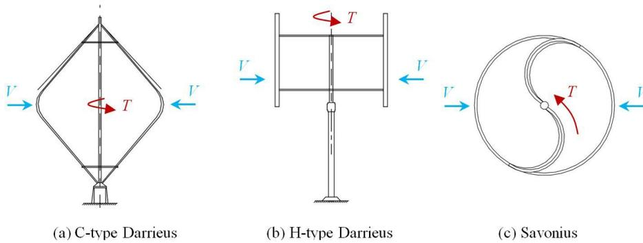
Figure 2 Typical Vertical Axis Wind Turbine configurations <sup>1</sup>
