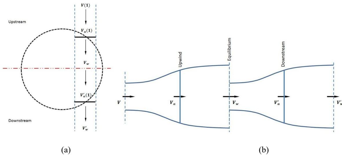
Figure 13 Schematic drawing of (a) double multiple streamtube model and (b) two actuator discs in tandem <sup>5</sup>
