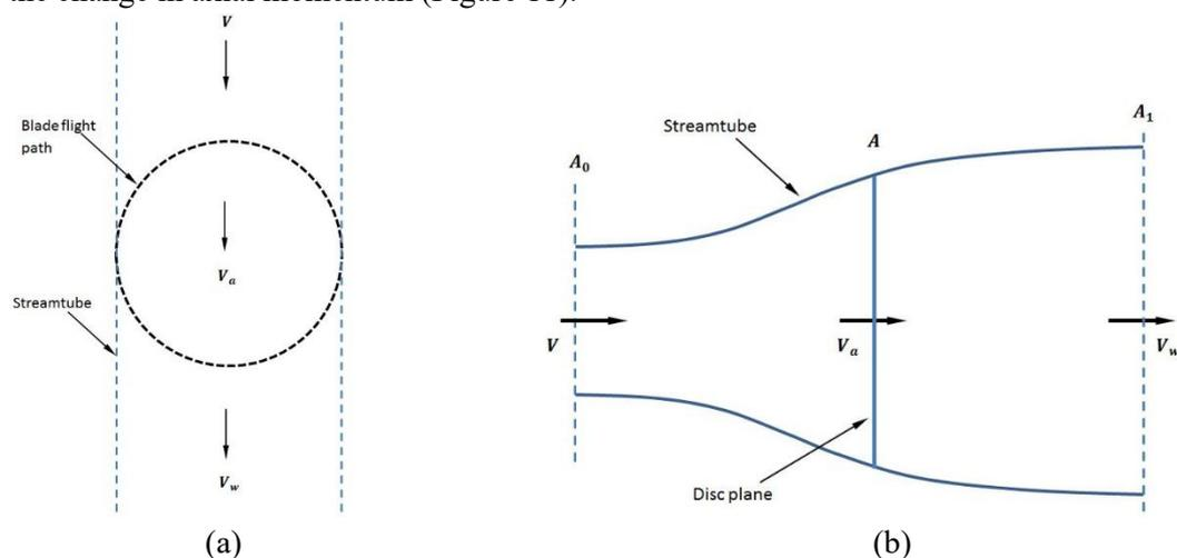
Figure 11 Schematic drawing of (a) single streamtube model and (b) actuator disc theory<sup>5</sup>
