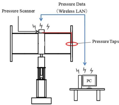
Figure 20 Schematic diagram of the pressure measurement principle <sup>178</sup>
