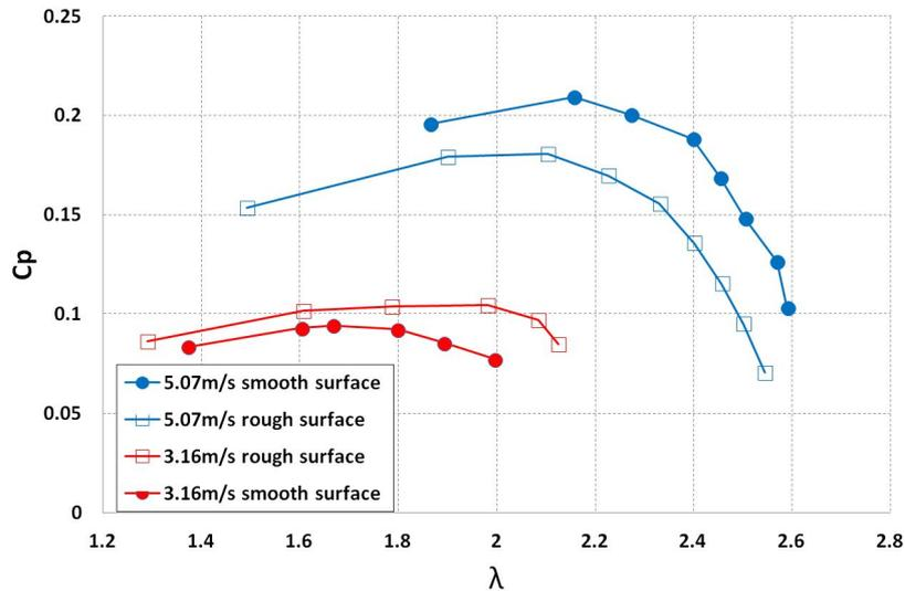
Figure 10 Turbine power output at different wind speed for smooth and rough blade surfaces<sup>37</sup>
