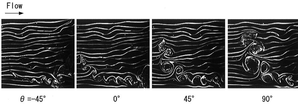
Figure 17 Flow visualization of dynamic stall of H-Darrieus wind turbine <sup>166</sup>
