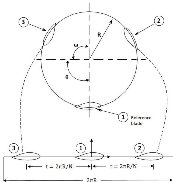
Figure 15 Cascade model configuration <sup>104</sup>
