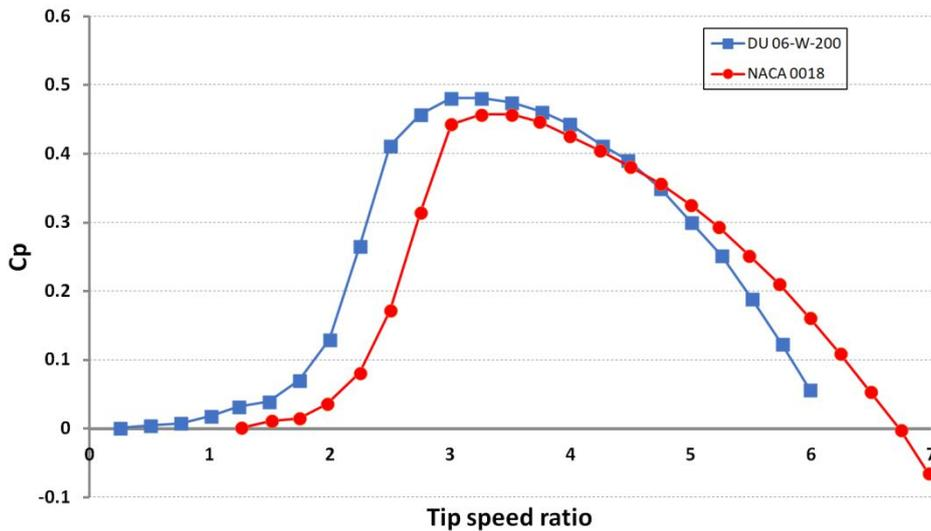
Figure 5 Turbine power coefficient with DU06W200 profile compared with NACA0018 profile<sup>61</sup>
