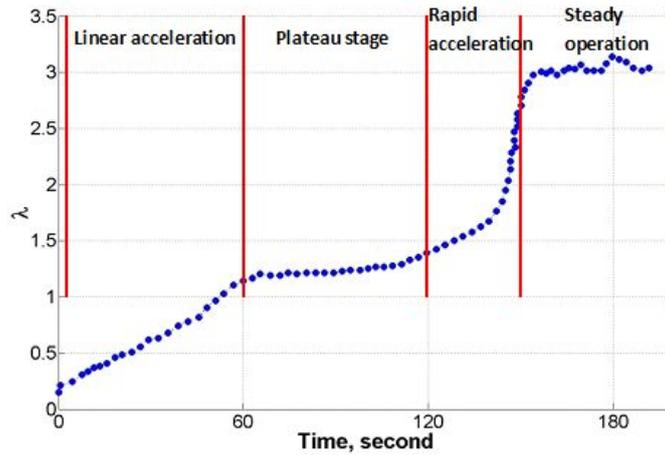
Figure 3 Measured H-Darrieus turbine starting behaviour from Hill et al.<sup>17</sup>.
