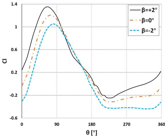
323 Figure 9 Blade lift coefficient versus azimuth angle for pitch angle of , and <sup>92</sup>.
