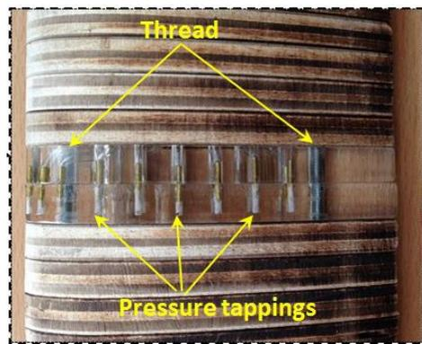
Figure 18 The NACA0021 blade with the pressure tapping section made from perspex<sup>5</sup>
