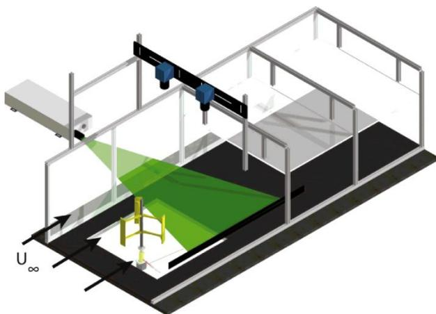
Figure 16 Schematic of typical PIV set-up<sup>167</sup>
