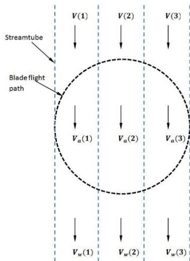
Figure 12 Schematic drawing of Multiple Streamtube model<sup>5</sup>
