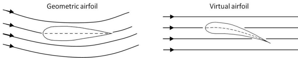
Figure 7 Schematic drawing of curvature effects for symmetric blades moving in a curvilinear flow <sup>71</sup>
