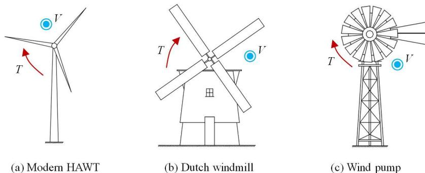
Figure 1 Typical Horizontal Axis Wind Turbine configurations <sup>1</sup>
