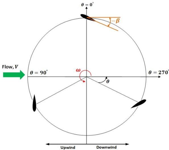
Figure 8 Definition of blade pitch angle <sup>5</sup>
