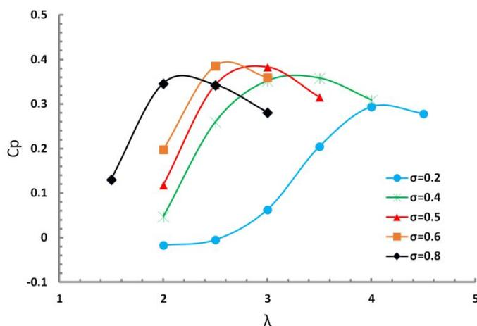
Figure 4 Effect of solidities on fixed pitch VAWT power curve performance<sup>42</sup>
