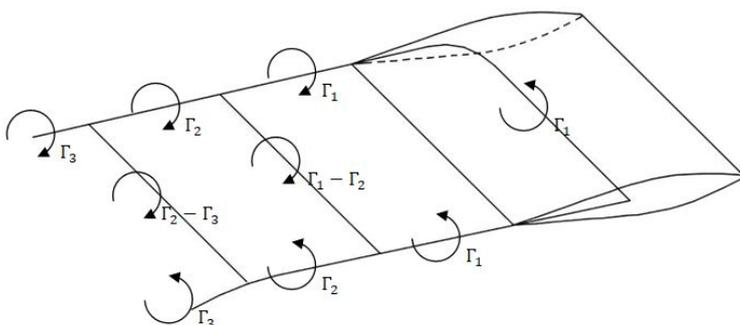
Figure 14 Vortex system for a single blade element <sup>104</sup>
