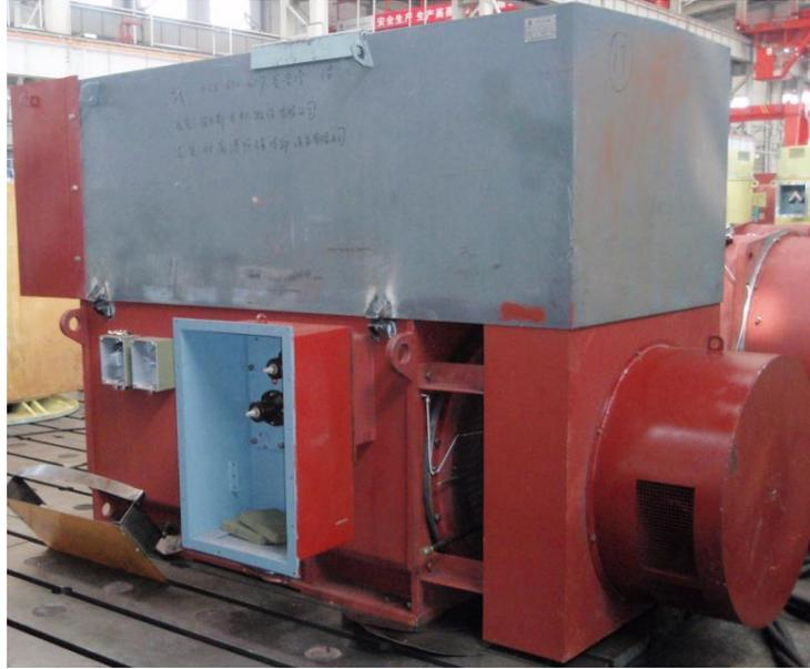
Fig.2 Compact high-voltage motor prototype
