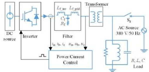
Fig. 11. Simulation platform
