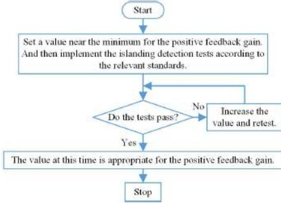
Fig. 1. A simple trial and error procedure
