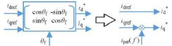
Fig. 4. Reformation of RCP method to SFS method
