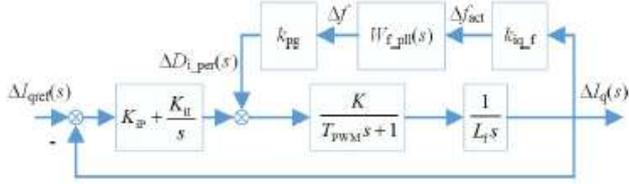
Fig. 8. Small signal model for the reactive current in an island condition
