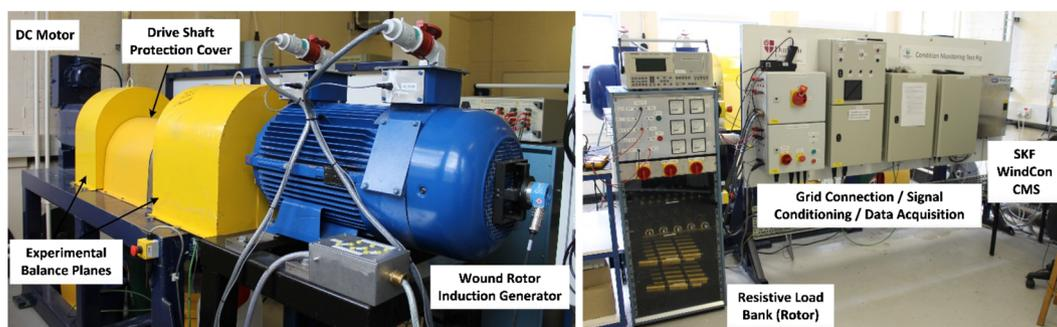
**FIGURE 3** Wind turbine condition monitoring test rig: main components, instrumentation, and control systems<sup>34</sup> [Colour figure can be viewed at [wileyonlinelibrary.com](http://wileyonlinelibrary.com)]
