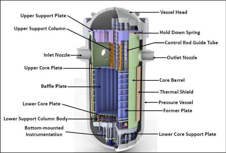
**Figure 1 - Illustration of Typical Pressurized Water Reactor Assembly**
