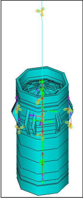
**Figure 2 - Illustration of System Finite Element Model**
