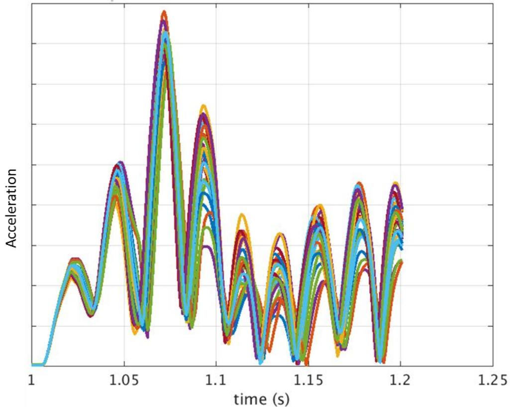
**Figure 5 - Acceleration Time Histories for RVCH lateral motion, where each line shows a different sample of the random parameters. Note that units are not provided due to information release restrictions.**
