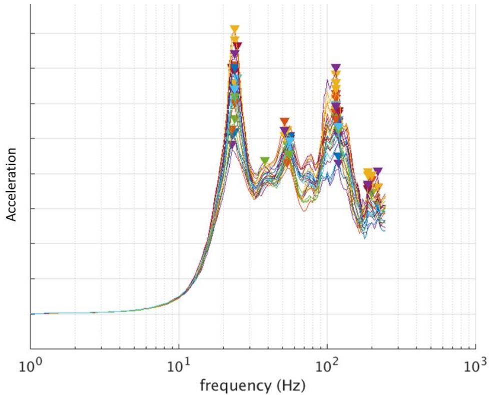
**Figure 6 - Acceleration Response Spectra Overlay of RVCH Lateral Motion, where each line shows a different sample of the random parameters. Note that units are not provided due to information release restrictions.**
