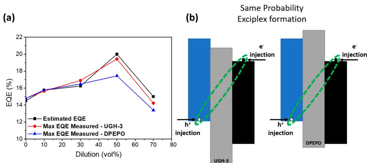
**Figure 5.** (a) Comparison between the measured maximum EQE values of OLED devices with different dilutions in UGH-3 and DPEPO, along with estimated EQE values calculated from UGH-3 nitrogen PLQYs. (b) Schematic representation of the exciplex formation mechanism under electrical excitation in OLED devices.
