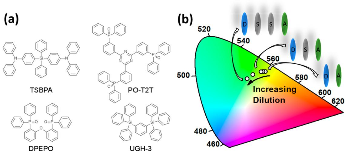
**Figure 1.** (a) Molecular structures of exciplex-forming molecules TSBPA and PO-T2T and the hosts molecules UGH-3 and DPEPO. (b) 1931 CIE chromaticity diagram schematically showing the blue shift of the exciplex emission with increasing dilution from the neat exciplex to 90 vol % UGH-3.
