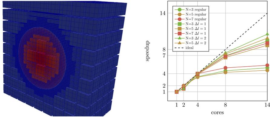
**Fig. 13.** Left: The TOV star setup showing two levels of adaptive mesh refinement along a sphere around the star. Right: Shared-memory scalability of the non-linear hybrid ADER-DG – FV implementation when running the TOV star example.
