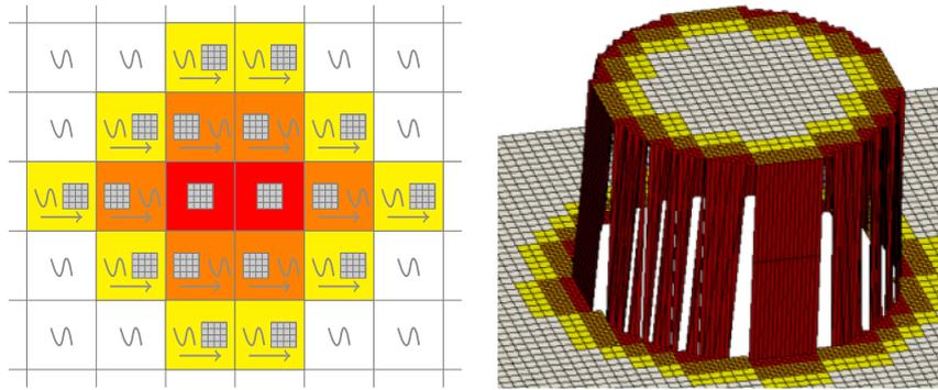
**Fig. 2.** Left: Limiter status stencil. Two FV cells (red) are surrounded by (ADER-)DG cells (white). Cells in the interface layers compute with FV and project to DG (orange) or with DG and project to FV (yellow). Right: The FV and DG subdomains are initialised along a discontinuity. (For interpretation of the references to colour in this figure legend, the reader is referred to the web version of this article.)
