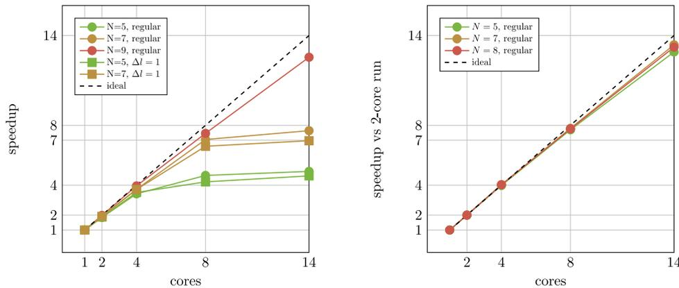
**Fig. 9.** Shared-memory scalability of the linear ADER-DG implementation on SuperMUC's Phase 2 when running the LOH.1 benchmark. Left: Curvilinear elements are used. Right: The diffuse interface method is used.
