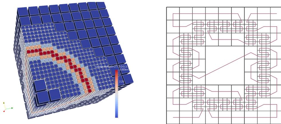
**Fig. 1.** Left: Adaptive Cartesian mesh in 3 dimensions. The FV limiter is active on the finest level. Right: Peano space-filling curve running through a 2D mesh that has a similar refinement pattern.
