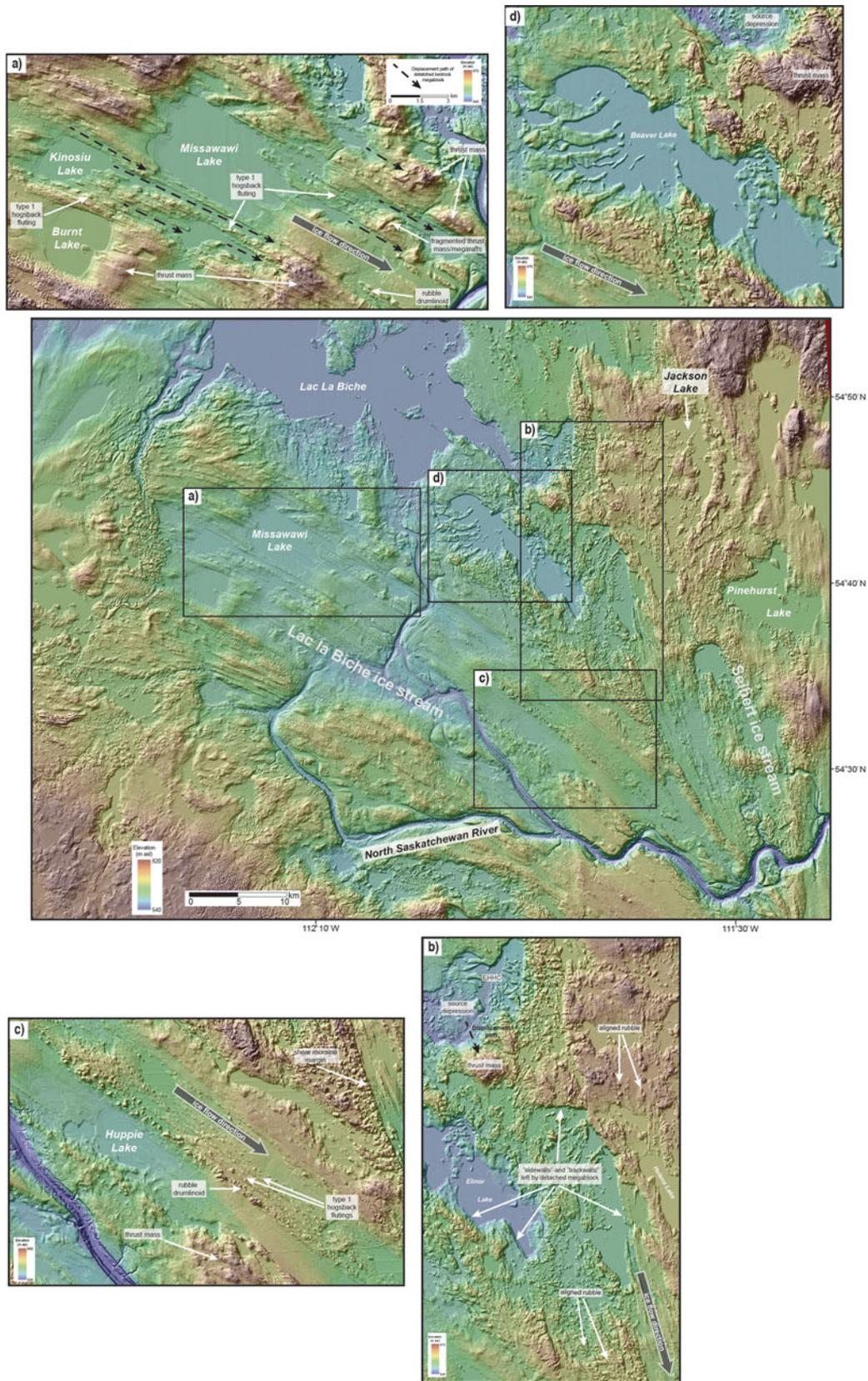
**Figure 9.** (color online) Annotated LiDAR digital elevation model of the glacial landforms in the area around Lac la Biche and Beaver Lake. Inset boxes show: (a) streamlined inner zone of the Lac la Biche Ice Stream trunk; (b) western boundary zone of the Seibert Ice Stream; (c) streamlined rubble of the inner zone of the Lac la Biche Ice Stream trunk; (d) the Beaver Lake en échelon hill-hole complex (EHC).
