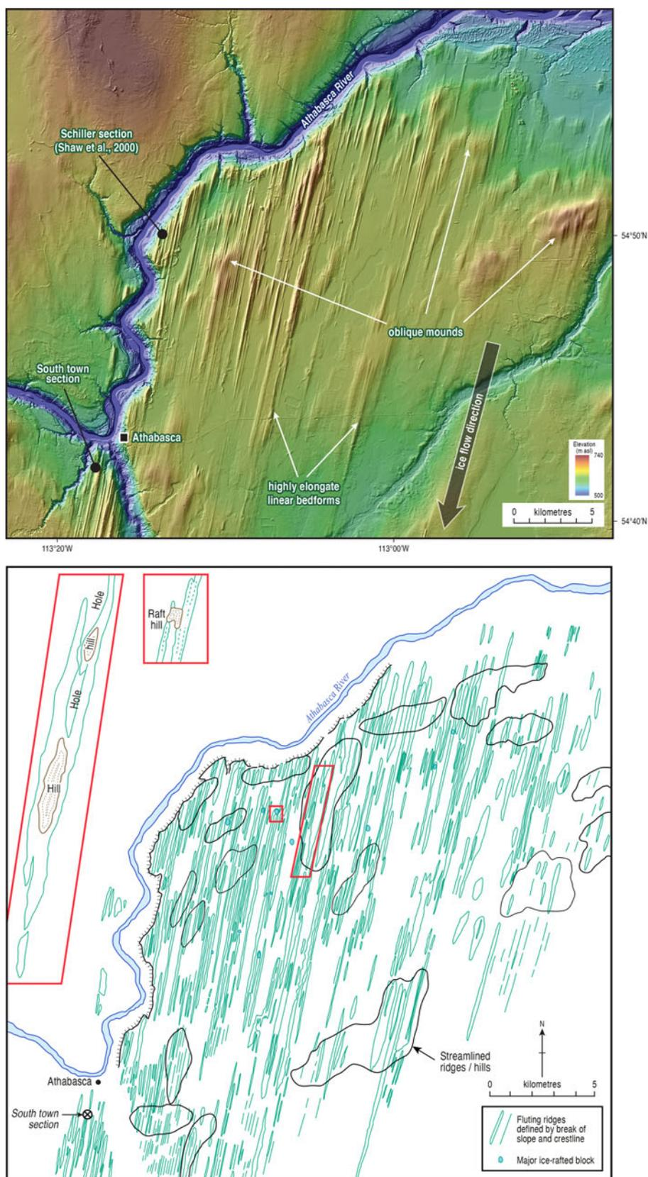
**Figure 3.** (color online) Annotated LiDAR digital elevation model (top) and geomorphology map (bottom) of the megafuting field located near the Athabasca townsite, showing the locations of exposures studied as well as that of Shaw et al. (2000).
