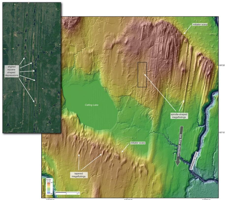
**Figure 4.** (color online) Annotated LiDAR digital elevation model of megafluting fields, drumlins, and initiator scarps near Calling Lake. The Google Earth image (inset) shows an enlarged area of the western flutings and illustrates examples of the chains of straight-sided depressions in the flat-floored grooves.
