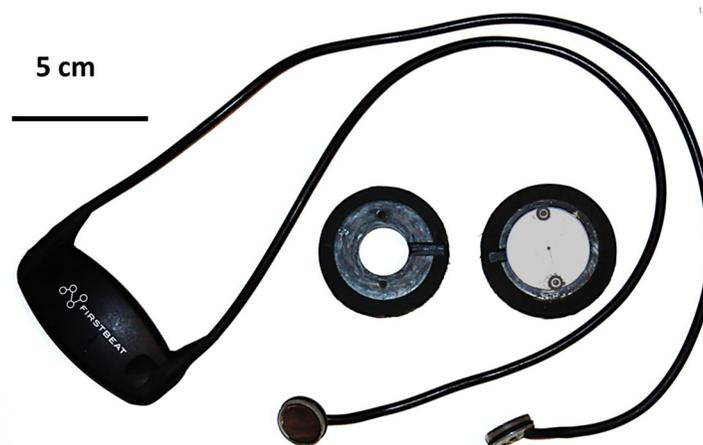
**Fig 1. Firstbeat™ transmitter and modified electrodes.** Image also shows the two attachment donuts, the right hand one with cover plate in place.
