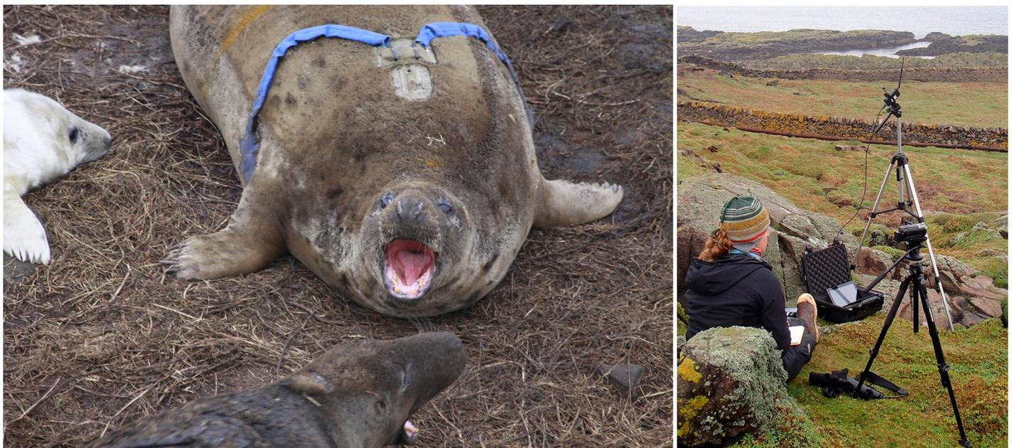
**Fig 2. The mounting of the Firstbeat™ transmitter and modified electrodes on an adult female grey seal.** Devices and cables were protected by nylon (blue and green in Fig 2A). Anterior of the centrally mounted heart rate transmitter is the accelerometer mounting (a). Data were transmitted to a receiving station located within line-of-sight at distances of up to 200 m from instrumented seals (b).
