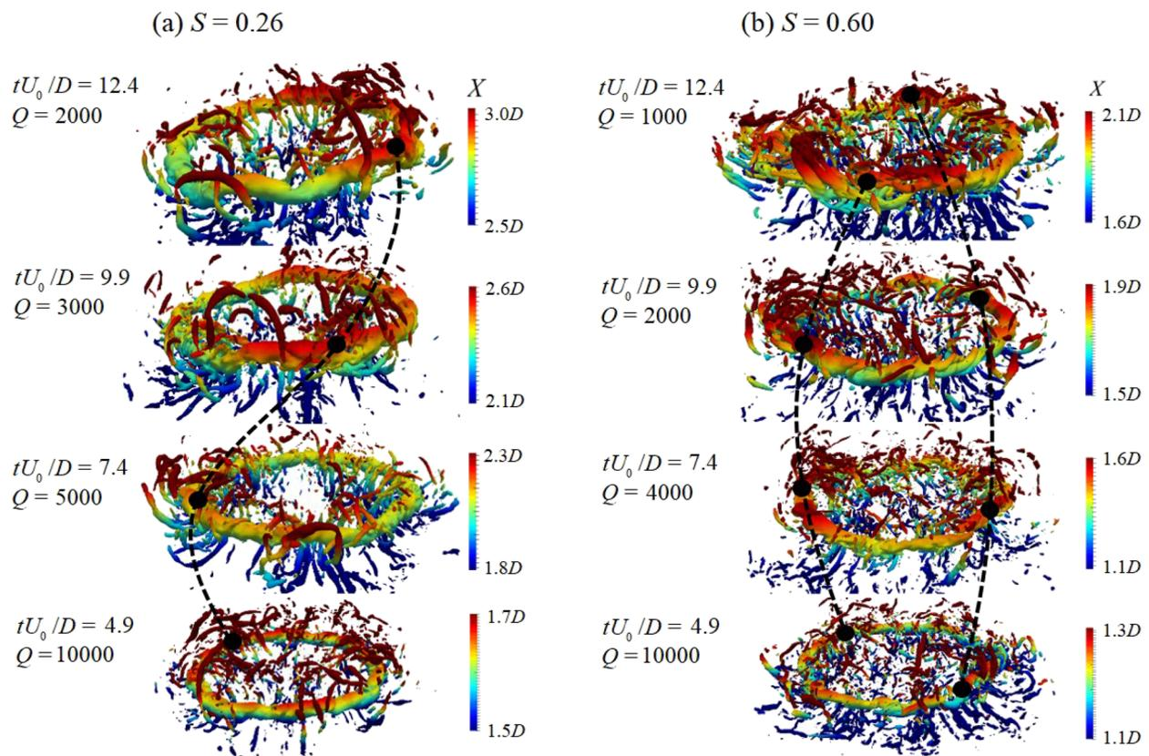
FIG. 16.  $m = 1$  (left) and 2 (right) modes observed in simulation results. Isosurfaces are colored by the axial coordinate value. (a) for  $S = 0.26$  and (b) for  $S = 0.60$ .
