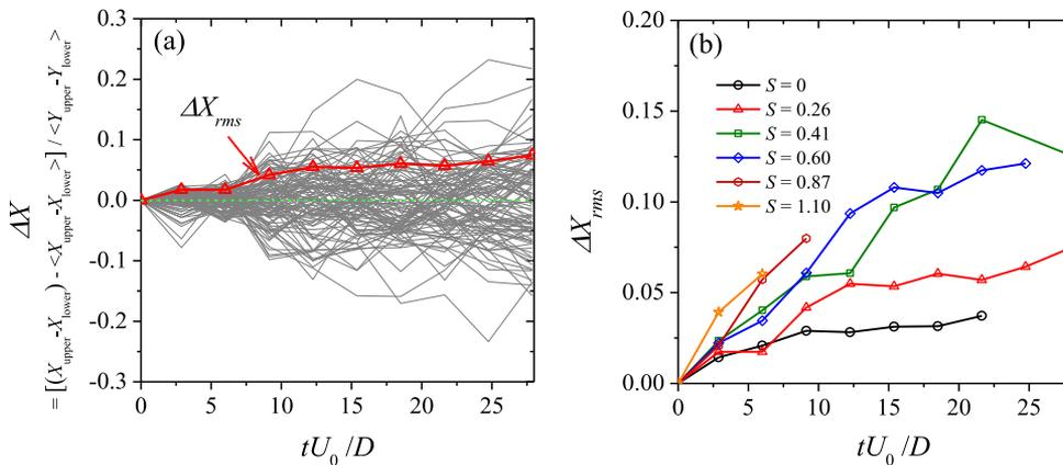
**FIG. 13.** Variation of the axial distances between the upper and lower core measured by planar-PIV. 100 realizations and the corresponding root-mean-squares of  $S = 0.26$  are plotted in (a), and the variation of the root-mean-squares for different  $S$  is plotted in (b).
