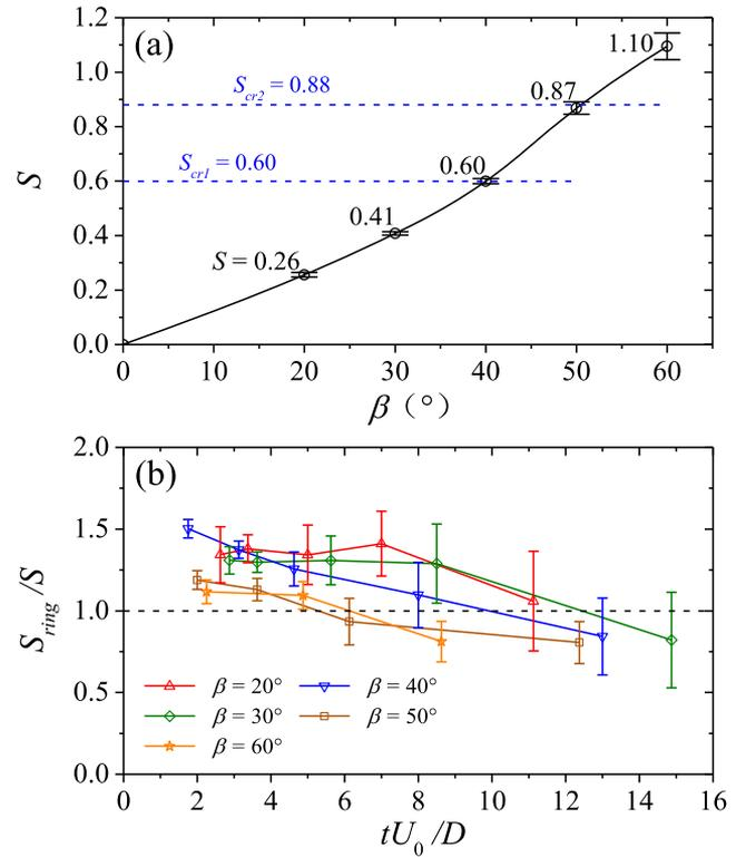
**FIG. 3.** Fully developed swirl numbers of each swirler geometry measured by planar-PIV at the steady state jet condition (a) and the dependence of the maximum sectional swirl numbers of the flow on the formation time measured by stereo-PIV (b). Error bars are determined using 100 repeated flow realizations.
