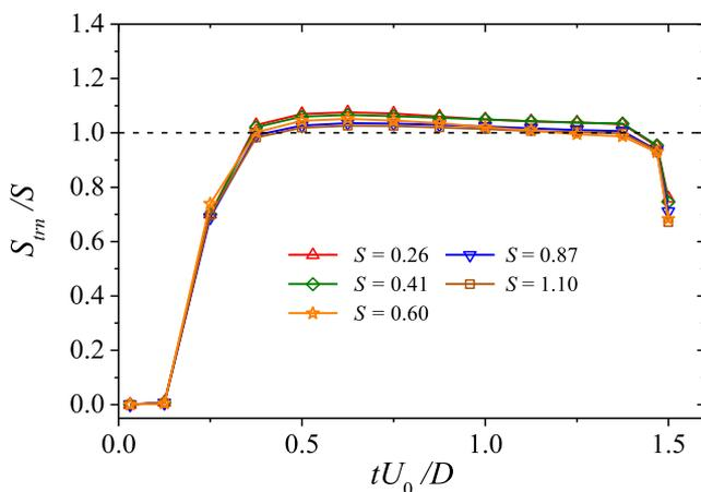
FIG. 6. The transient swirl number at the swirler exit calculated using the simulation results.
