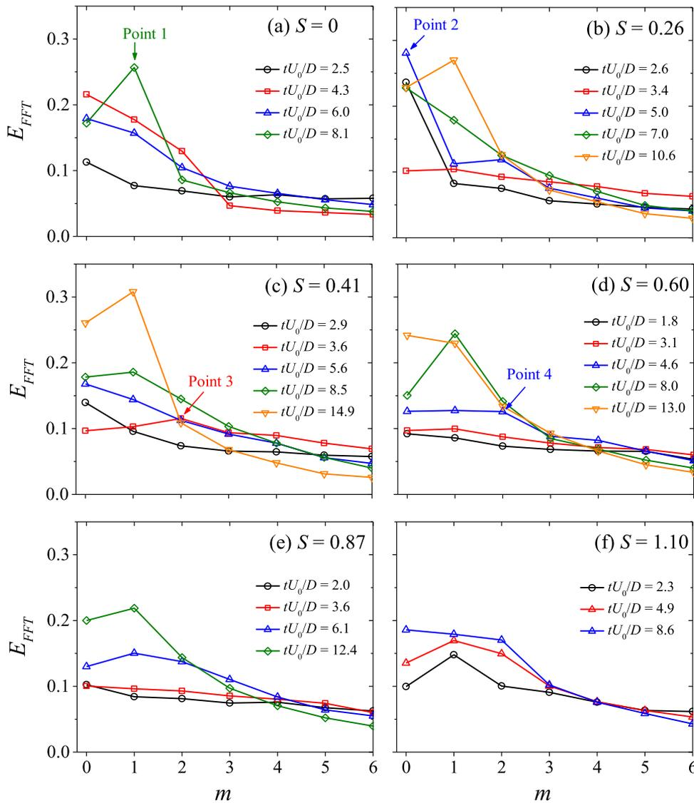
**FIG. 14.** Energy of the Fourier modes at each azimuthal wavenumber calculated using stereo-PIV results. [(a)–(f)] for  $S = 0, 0.26, 0.41, 0.60, 0.87,$  and  $1.10,$  respectively.
