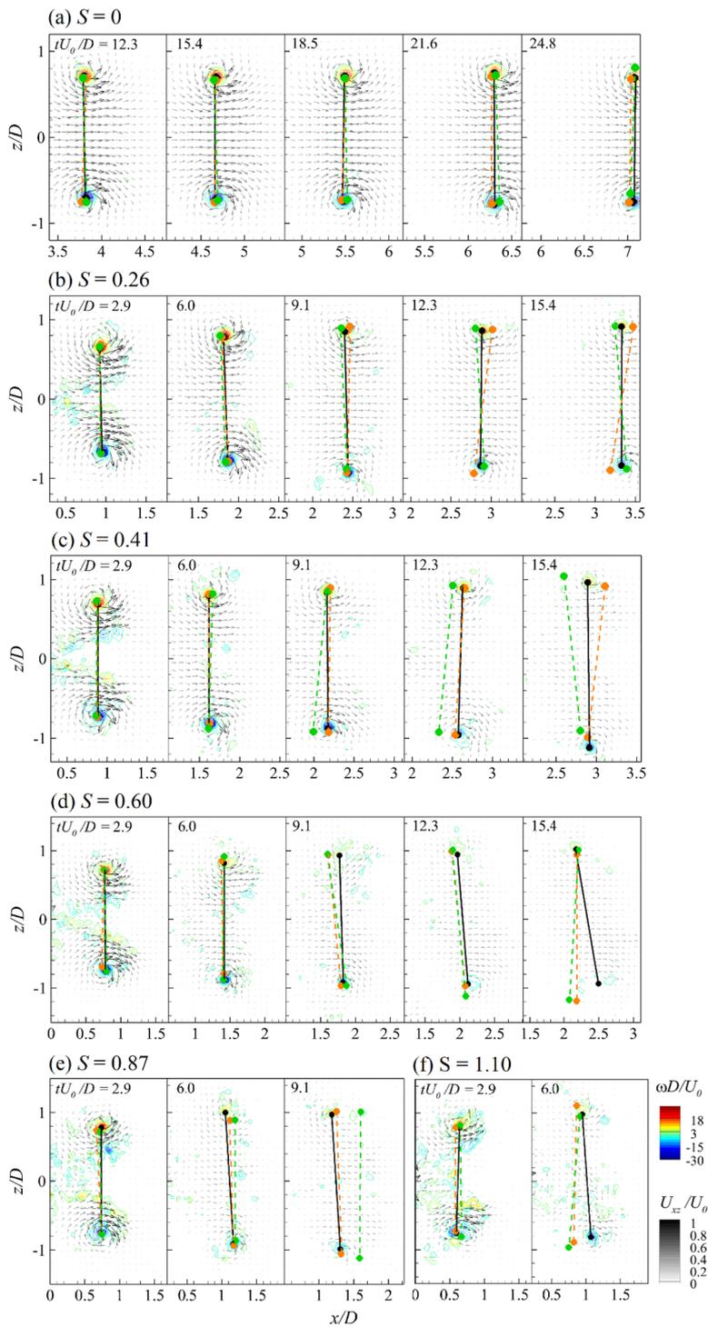
FIG. 11. Instantaneous ring core location for three independent realizations (denoted by black, green, and orange dots and bars) determined by planar-PIV. [(a)–(f)] for  $S = 0, 0.26, 0.41, 0.60, 0.87,$  and  $1.10,$  respectively.
