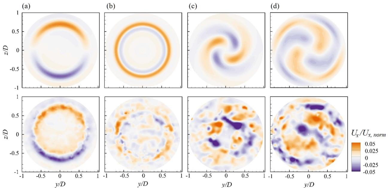
**FIG. 15.** Azimuthal modes (upper) captured using stereo-PIV measurements and the instantaneous fluctuating axial velocity (lower) at the points marked in Fig. 13. Point 1 (a), point 2 (b), point 3 (c), and point 4 (d). Velocity is normalized by the matrix norm  $U_{x, norm}$ .
