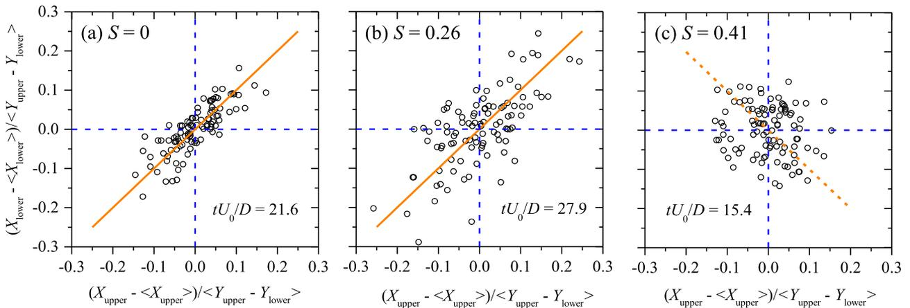
**FIG. 12.** Coordinate maps of the upper and lower parts of the ring cores measured by planar-PIV. Each data point represents a realization. [(a)–(c)] for  $S = 0, 0.26,$  and  $0.41,$  respectively.
