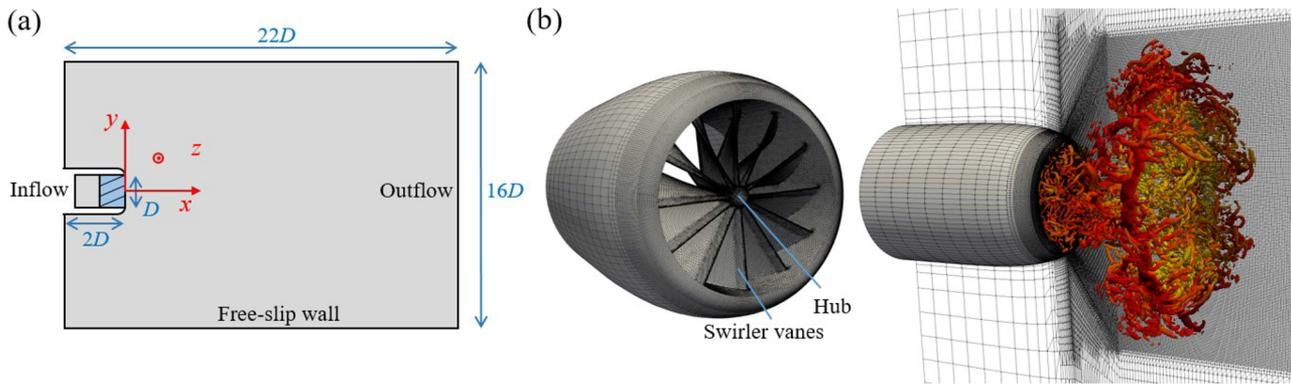
**FIG. 2.** (a) The schematic diagram of the numerical setups (side view) and (b) the nozzle geometry with  $\beta = 40^\circ$  and computational grid (isosurface shows the ring structure at  $tU_0/D = 5$ ).
