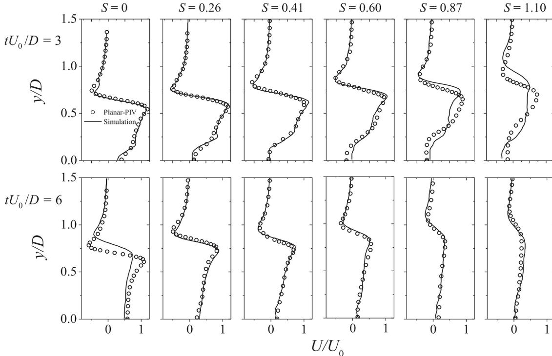
**FIG. 5.** Comparison of axial velocity distributions of dynamic DDES and planar-PIV results at  $tU_0/D = 3$  (upper row) and 6 (lower row).
