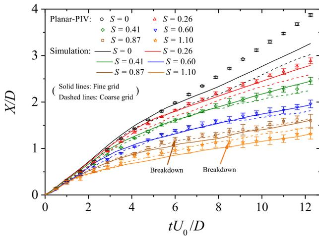
**FIG. 4.** Axial trajectories of the vortex ring core: comparison of the present dynamic DDES results with the planar-PIV measurements. Error bars are determined using 20 repeated flow realizations (fine grid: 2 levels of refinement; coarse grid: 1 level of refinement).
