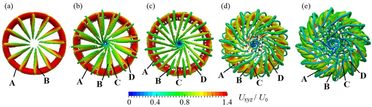
**FIG. 8.** Three-dimensional structures of the primary vortex ring and secondary vortices for  $S = 0.60$  at  $tU_0/D =$ : (a) 0.25, (b) 0.38, (c) 0.50, (d) 1.13, and (e) 1.50. Simulation results:  $U_{xyz} = \sqrt{U_x^2 + U_y^2 + U_z^2}$  denotes the velocity amplitude in the three-dimensional domain. Different vortical structures are named as follows: **A**, primary vortex ring; **B**, starting wake vortices; **C**, vane boundary vortices; and **D**, inner boundary vortices.
