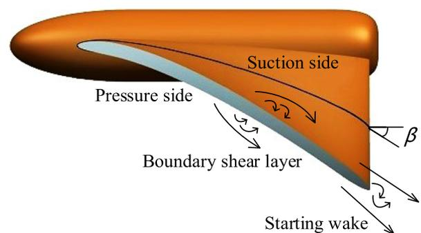
FIG. 7. Schematic diagram of the starting wake and vane boundary vortices generation.
