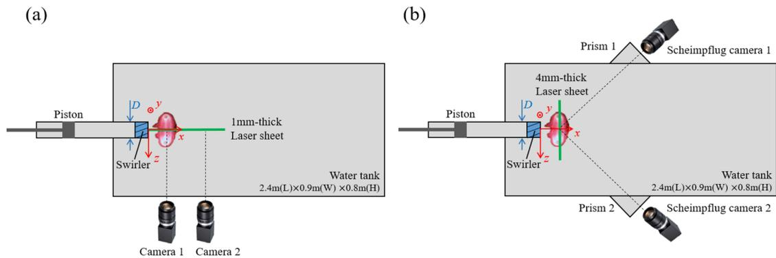
FIG. 1. The schematic diagram (top view) of (a) the planar-PIV and (b) stereo-PIV measurements.
