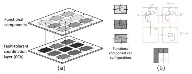
FIGURE 9. Illustration of resilient logic implemented using a CCA coordination layer and functional logic layer. (a) arrangement of coordination and function layers along with example component cell configurations; (b) Illustrative example configuration for combinatorial logic adder with simple CCA coordination pattern.
