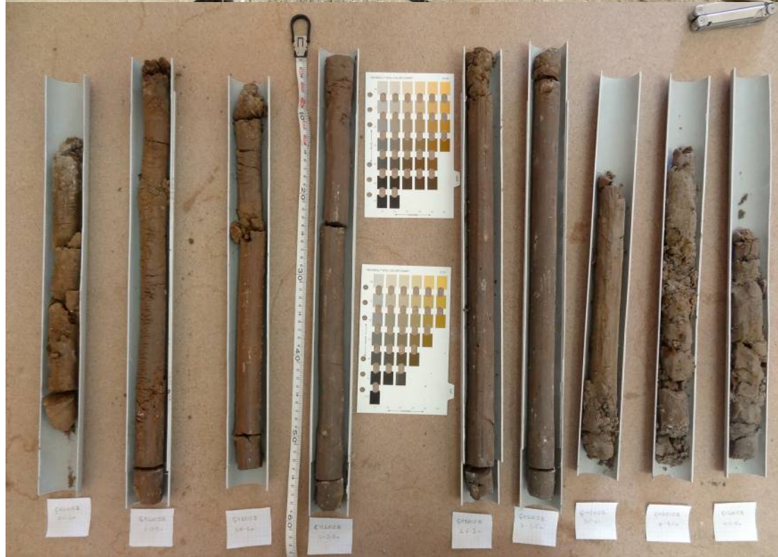
Figure 3. Sediment coring during the 2015 field campaign: (a) a core starting to be drilled. The screw core is taken down to the level of interest, and then a core tube (seen lying on the frame in the foreground) is pushed into the sediment to obtain a core sample; and (b) sediments recovered from core 2015/B (see fig. 6 for location).
