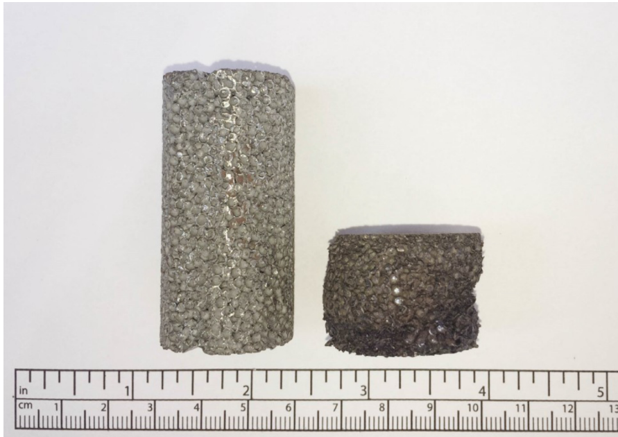
Fig. 9. (left) HS steel foam specimen before testing, and (right) HS steel foam specimen after testing at 300 °C following 30 min of exposure. Discoloration of the heated specimen indicated formation of a blue oxide film on the surfaces of the spherical shells. (For interpretation of the references to colour in this figure legend, the reader is referred to the web version of this article.)
