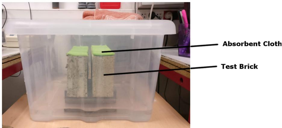
**Fig. 3.** Test setup for contact tests.
