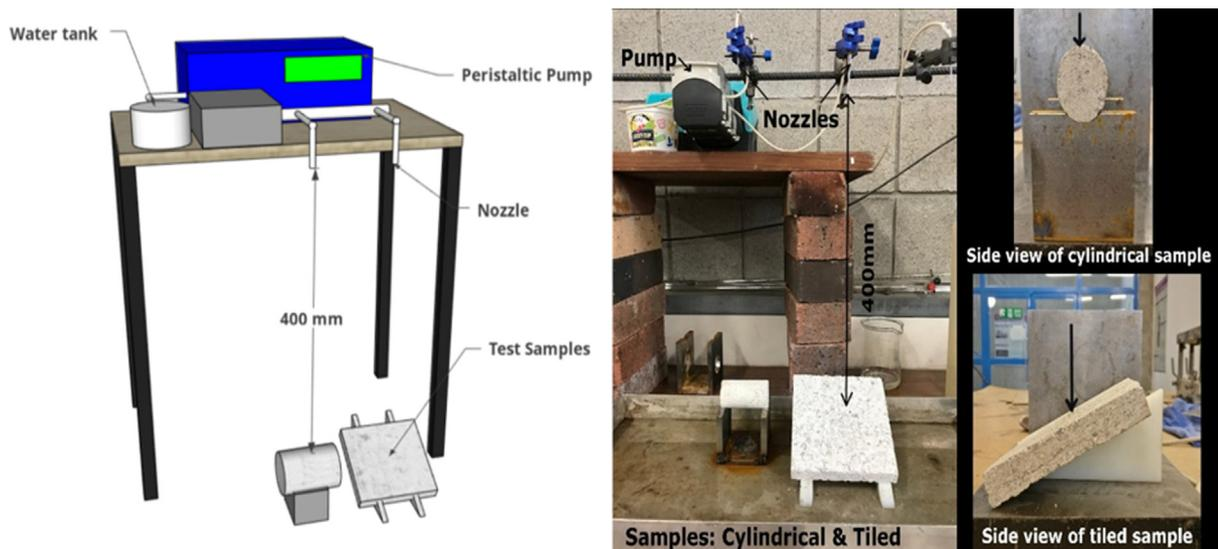
Fig. 10. Test setup for Geelong erosion test.
