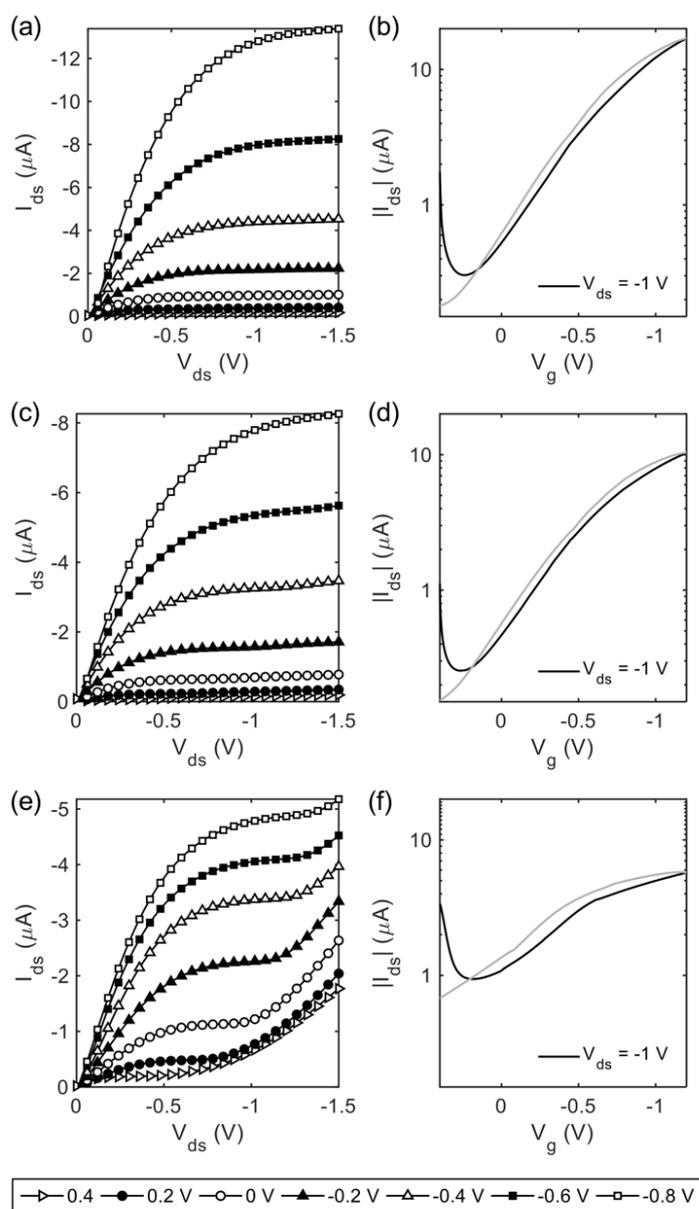
**Figure 3.** Output and transfer characteristics for HIFETs gated by PEDOT:PSS films deposited from (a,b) 100%, (c,d) 25% and (e,f) 6% of the stock PEDOT:PSS dispersion. The legend below indicates gate voltages for the output curves. Black and grey lines in transfer curves indicate forward and reverse sweeps, respectively.
