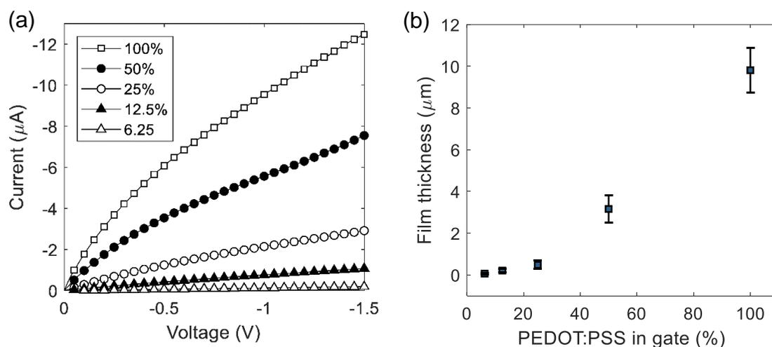
**Figure S1:** (a) Current-voltage relationship for PEDOT:PSS films deposited from dispersions of varied concentration. (b) Plot showing the relationship between thickness of PEDOT:PSS films and the concentration of PEDOT:PSS, expressed as a percentage of the stock solution. Film thickness is measured by stylus profilometry.
