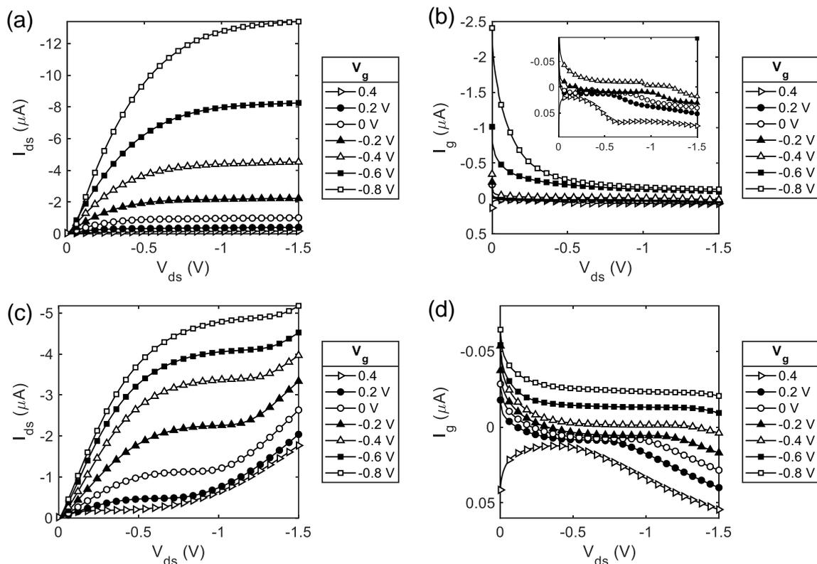
**Figure S7:** Figures plotting output characteristics, and gate current, measured simultaneously for, (a,b) a standard HIFET (100% PEDOT:PSS gate) and (c,d) a HIFET with a poorly conducting gate (6.25% PEDOT:PSS). Gate current changes dynamically with drain-source voltage.
