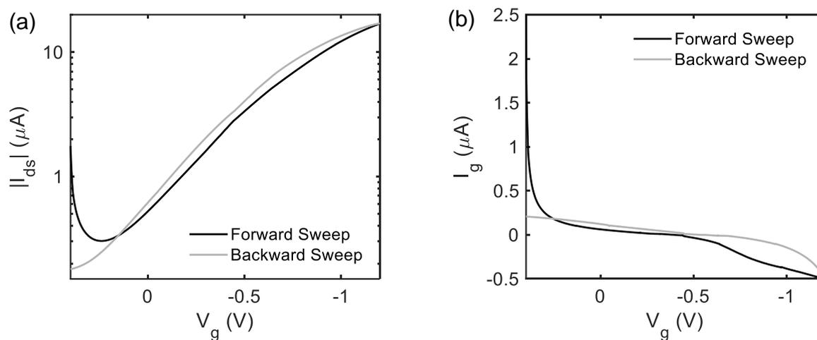
**Figure S6:** Figures plotting (a) transfer characteristics, and (b) gate current, measured simultaneously (at  $V_{ds} = -1\text{V}$ ) for a standard HIFET (100% PEDOT:PSS gate). Gate current changes dynamically with gate voltage.
