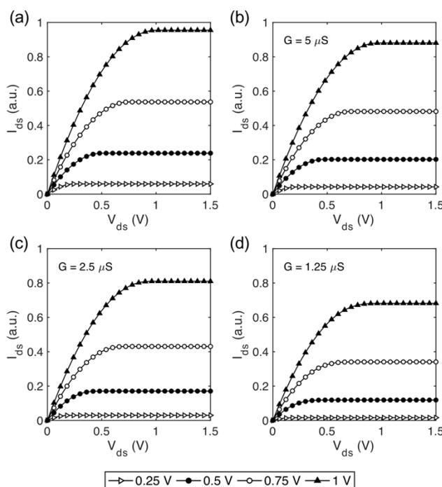
**Figure 5.** Simulated output curves, using (a) the standard gradual channel approximation, (b,c,d) modified gradual channel approximation with decreasing gate conductance ( $G$ ), corresponding to increased  $\beta$ .
