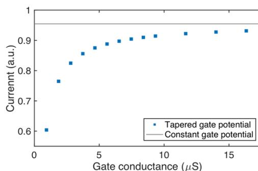
**Figure 6.** Simulated saturation current  $I_{\text{sat}}$  at  $V_g = -1\text{V}$  for the modified gradual channel approximation with gate conductance. Grey line shows the result for the standard gradual channel approximation.
