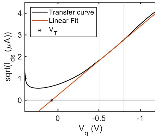
**Figure S4:** Figure showing the extraction of the threshold voltage for a standard HIFET (100% PEDOT:PSS gate). The square root of  $I_{ds}$  is plotted with  $V_g$  and a straight line is fitted to the region enclosed by the vertical grey lines, which is approximately linear. The threshold voltage is the point at which the fitted line crosses the x-axis.
