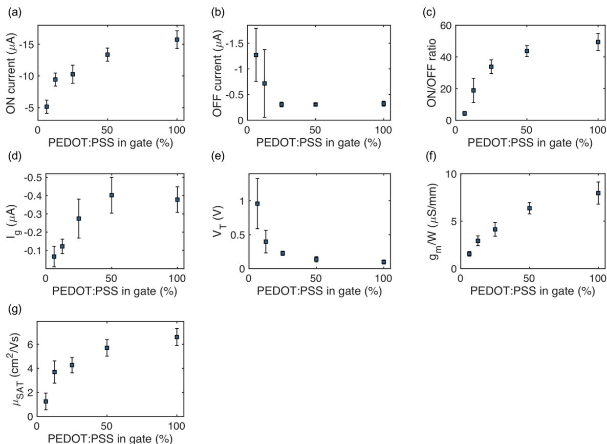
**Figure 4.** Plots showing the variation of key figures of merit with the amount of PEDOT:PSS in the gate. Figures of merit shown are the (a) ON current, (b) OFF current, (c) ON/OFF ratio, (d) gate current at  $V_g = -1$  V and  $V_{ds} = -1$  V, (e) threshold voltage, (f) transconductance, and (g) apparent saturation mobility.
