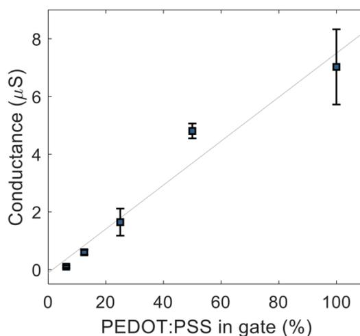
**Figure 2.** Conductance of PEDOT:PSS gates with dilution.
