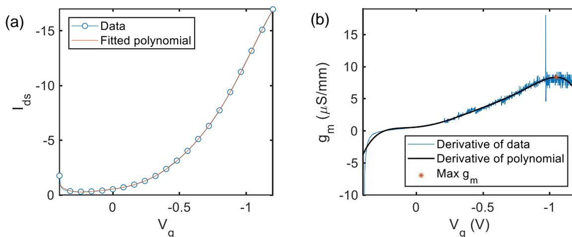
**Figure S5:** Figures showing the extraction of the transconductance for a standard HIFET (100% PEDOT:PSS gate). (a) The transfer curve is plotted and a polynomial is fitted. (b) The first derivative of the fitted polynomial is plotted alongside an approximate derivative of the measured data set. The polynomial follows the data reasonably well, but without the noise. The maximum transconductance is extracted from the derived polynomial.
