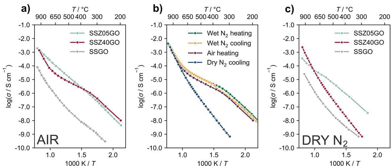
**Figure 2.** Conductivity as a function of temperature for SSZ40GO and related compounds: (a) comparison of conductivities in air for the different compounds, (b) conductivity under different atmospheres for SSZ40GO, and (c) comparison between conductivities in dry nitrogen for the different compounds. Data shown for SSGO and SSZ05GO are from both heating and cooling cycles.
