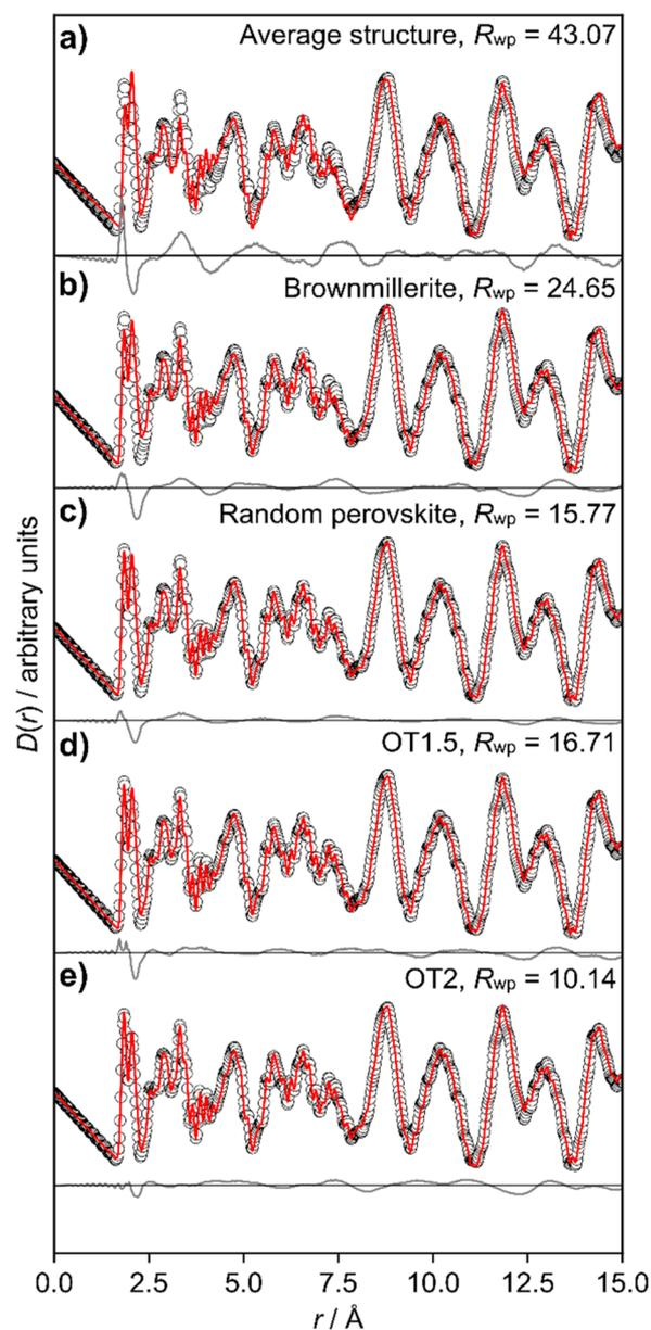
**Figure 6.** Fit of various local structure models (red curve) to the measured PDF (black markers) data of SSZ40GO. Difference curves are shown in gray. The  $R_{wp}$  values given are calculated for  $1.5 \text{ \AA} \leq r \leq 8 \text{ \AA}$  to reflect the fit to the local structure.
