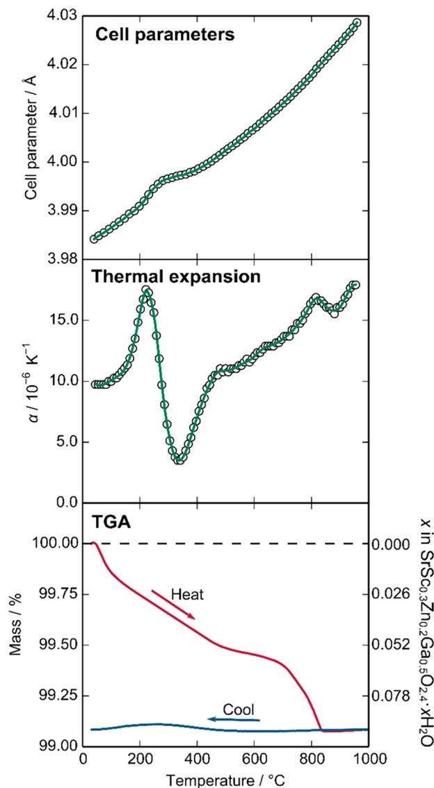
**Figure 3.** SSZ40GO cell parameter evolution with temperature from variable temperature X-ray diffraction (top panel) and derived thermal expansion ( $da/dT$ ) (middle). Thermogravimetric analysis over the same temperature range (bottom) on both heating and cooling cycles. Cell parameters on cooling are shown in the Supporting Information.
