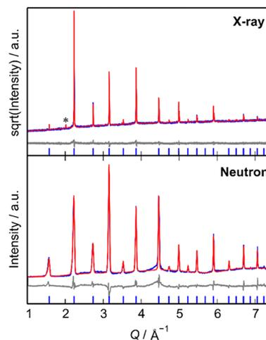
**Figure 1.** Rietveld fits of a simple  $Pm\text{-}3m$  perovskite model against the room temperature X-ray (top) and neutron (bottom) data for SSZ40GO. Blue, red, and gray curves show the observed, calculated, and difference curves, respectively. Blue tick marks indicate the expected peak positions. The peak highlighted with an asterisk is a result of  $W\text{La}$  incident X-ray contamination. X-ray data are shown on a square root scale to emphasize weaker features.
