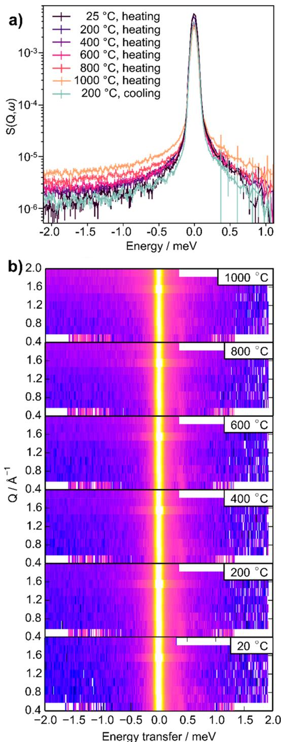
**Figure 4.** (a) Plot of the scattering function  $S(\omega)$  at  $Q = 1.92 \text{ \AA}^{-1}$  showing the QENS broadening of the elastic peak. (b) Color maps of  $S(Q, \omega)$  at different temperatures to show the evolution of the QENS broadening at high temperatures and that this is enhanced at high  $Q$ .
