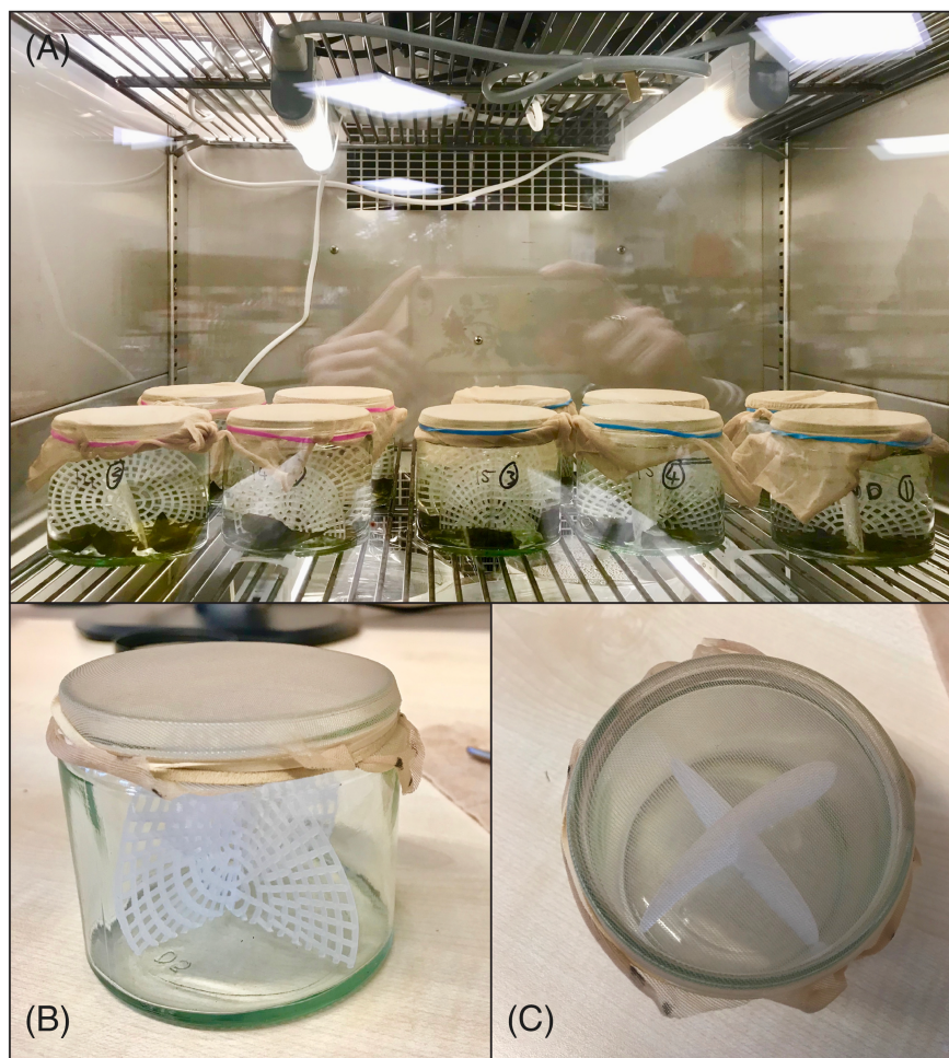
FIGURE 2 Photographs of the experimental jars used to culture the macroalgae tips in this study. A, The position of the jars in the incubator during the experiment. B, Side view of a jar with plastic mesh to separate macroalgal samples. C, Aerial view of a jar with plastic mesh and stocking material to allow atmospheric exchange and light penetration; in Gröcke et al. 7 the solid plastic lids were placed loosely on top which would have caused reduced light intensity [Color figure can be viewed at wileyonlinelibrary.com ]
