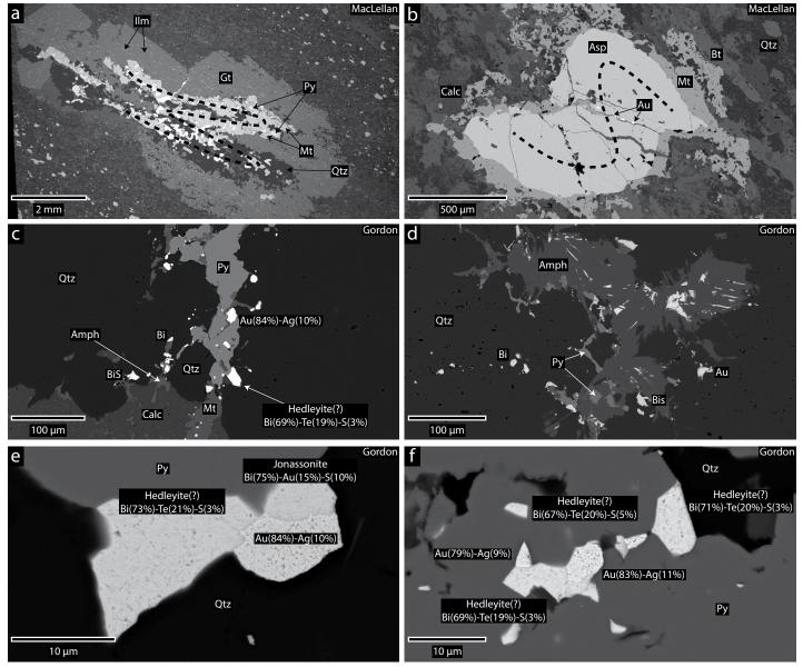
Scanning electron microscope (SEM) backscattered electron (BSE) images of gold ore zones
