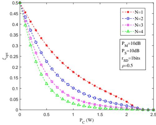
Fig. 1.  $\xi_{opt}$  versus  $P_C$  for different number of relays with  $P_M = 10\text{dB}$ ,  $P_S = 10\text{dB}$ ,  $\rho = 0.5$ ,  $r_{SD} = 1\text{bits}$ ,  $\sigma_S^2 = \sigma_{R_k}^2 = \sigma_D^2 = 1$ , and  $|h_{R_k S}|^2 = 1$ .
