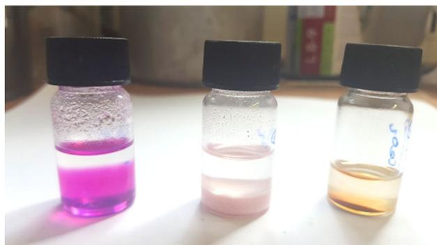
**Fig. 9** Photograph showing colour change on exposure of different oxide supports to and adsorption of the Hammett indicator methyl red in toluene solution: silica (left); titania (middle); ceria (right)
