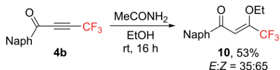
Scheme 9. Reaction of \text{CF}_3 -ynone 4b with ethanol.
