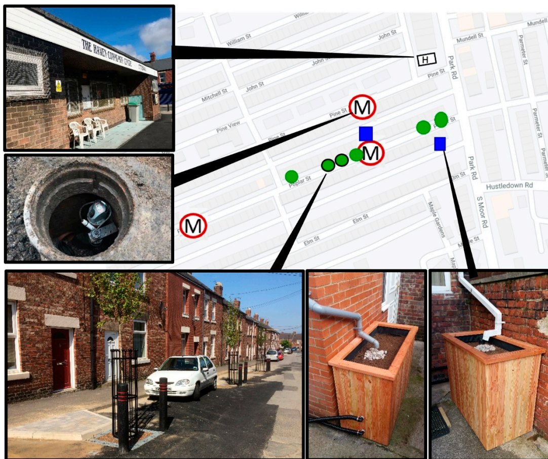
Figure 3. The location of three monitoring points (M), two rear yard planters (blue squares), four street trees (green circles) and two sustainable drainage systems (SuDS) tree pits (green circle with black edge) on Pine Street and Poplar Street (not to scale). The dashboard interface was installed in The Haven Community Centre (H).
