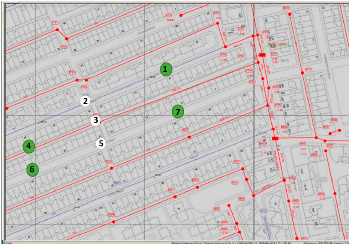
Figure 6. Locations for monitoring equipment in South Moor’s sewer network following inspection in late February 2018. Green dots show manholes suitable for installation of sensor, white dots show manholes not used in this study. Red lines highlight foul or combined sewers, and blue lines show surface water sewers. The position of private drains and sewers are not shown.
