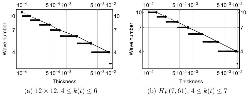
**Fig. 11.** Asymptotic analysis:  $k(t)$  and trend line; hole coverage 12%;  $t \in [10^{-4}, 10^{-2}]$ , uniform logarithmic scale with 100 samples. The rate in Table 1 is computed in the interval indicated with a solid line and in the caption, dashed line represents the perturbed part.
