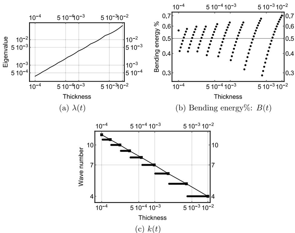
**Fig. 6.** Reference asymptotic analysis:  $t \in [10^{-4}, 10^{-2}]$ , uniform logarithmic scale with 100 samples. Observed rates:  $\lambda(t) \sim t$ ;  $k(t) \sim t^{-1/4}$ ;  $B(t) \rightarrow 1/2$ .
