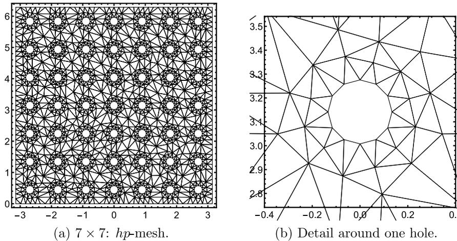
Fig. 5. Typical mesh configuration. In the detail, the hole is programmatically mapped to be circular in the assembly of the system. In the simulations the boundaries at  $x_1 = \pm\pi$  are clamped, holes are free, and  $x_2 = 0$  and  $x_2 = 2\pi$  are periodic.
