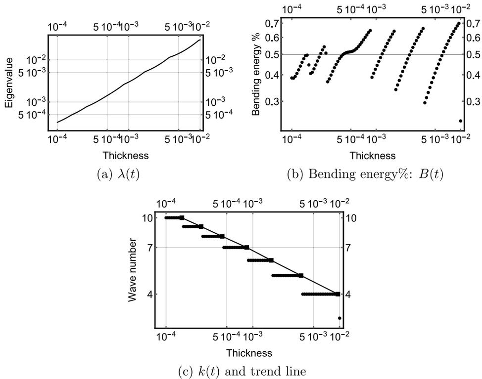
**Fig. 8.** Asymptotic analysis:  $15 \times 15$  regular grid; hole coverage 12%;  $t \in [10^{-4}, 10^{-2}]$ , uniform logarithmic scale with 100 samples. Observed rates:  $\lambda(t) \sim t$ ;  $k(t) \sim t^{-1/4}$ ,  $k(t) \leq 7$ . Notice that the width of the interval of thicknesses at  $k = 7$  extends below  $t = 5 \times 10^{-4}$ . Again, behaviour of  $B(t)$  changes at  $k = 7$ .
