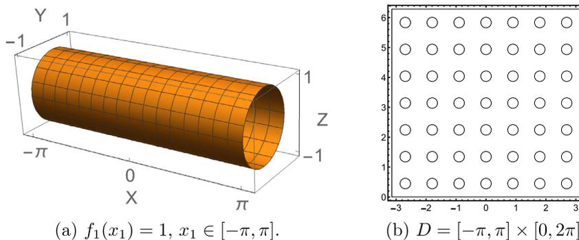
**Fig. 2.** Parabolic shell of revolution and the corresponding computational domain with a  $7 \times 7$  regular perforation pattern with 12% hole coverage. For free vibration the boundaries at  $x_1 = \pm\pi$  are clamped, holes are free, and  $x_2 = 0$  and  $x_2 = 2\pi$  are periodic.
