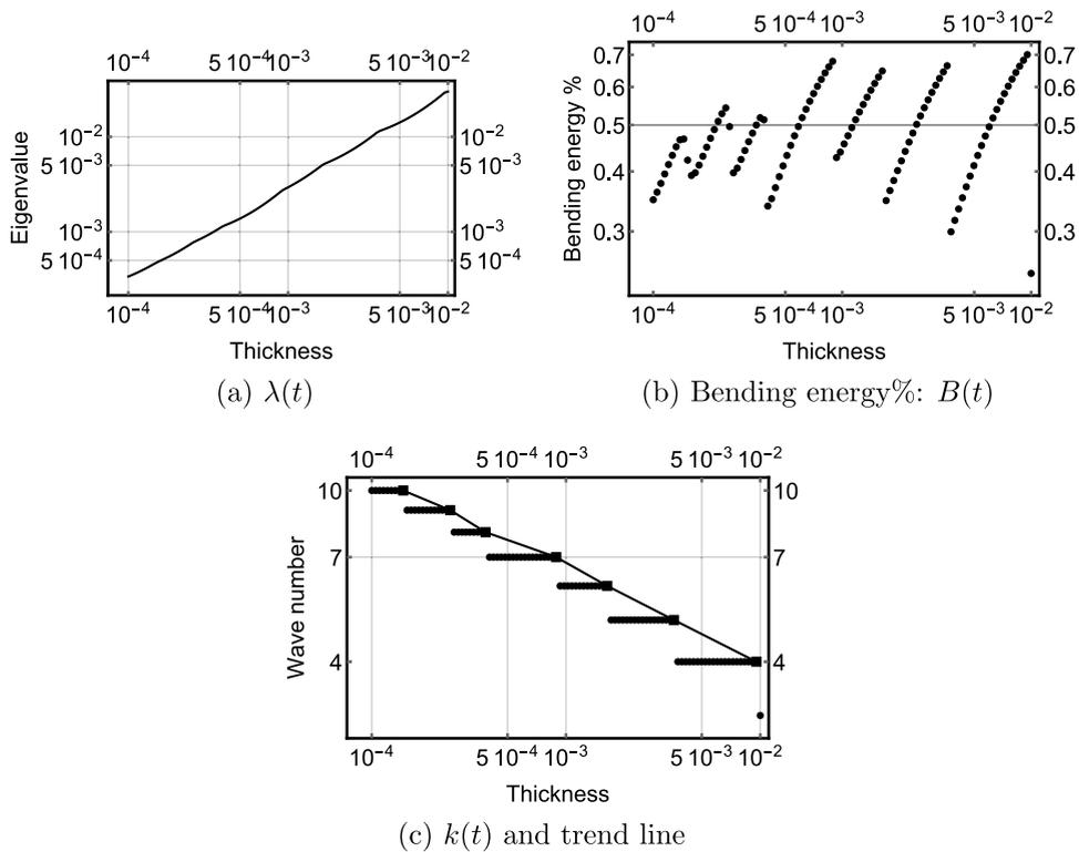
**Fig. 7.** Asymptotic analysis:  $14 \times 14$  regular grid; hole coverage 12%;  $t \in [10^{-4}, 10^{-2}]$ , uniform logarithmic scale with 100 samples. Observed rates:  $\lambda(t) \sim t$ ;  $k(t) \sim t^{-1/4}$ ,  $k(t) \leq 7$ . Notice the width of the interval of thicknesses at  $k = 7$ . Behaviour of  $B(t)$  changes at  $k = 7$ .
