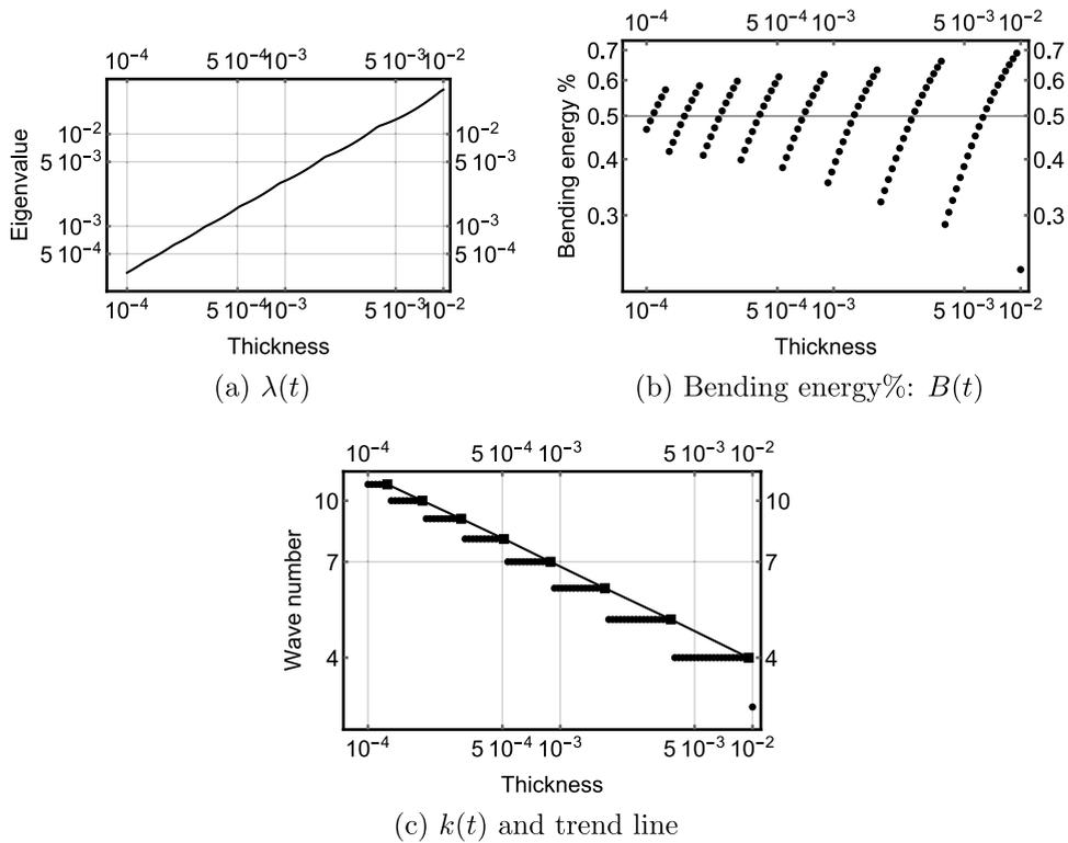
**Fig. 9.** Asymptotic analysis:  $30 \times 30$  regular grid; hole coverage 12%;  $t \in [10^{-4}, 10^{-2}]$ , uniform logarithmic scale with 100 samples. Observed rates:  $\lambda(t) \sim t$ ;  $k(t) \sim t^{-1/4}$ . Notice that the width of the interval of thicknesses at  $k = 7$  does not extend below  $t = 5 \times 10^{-4}$ . Within the parameter range  $B(t) \rightarrow 1/2$ .
