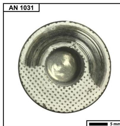
**Supplementary Figure 15** | Top view of the bottom cylinder (static) with the sheared sample ( $v = 0.58\text{ ms}^{-1}$ ). Samples commonly split along mirror-like surfaces (in the case of AN 1031, within the PSZ, see Supplementary Figure 6).
