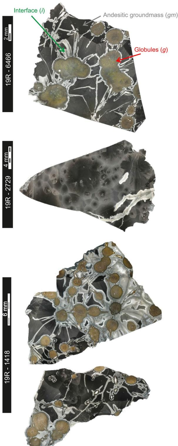
**Fig. 2** Overview images of samples 19R-1418, 19R-2729 and 19R-7274. Optical microscopy images taken under dark-field illumination were combined to create this overview. All samples exhibit globules surrounded by an andesitic groundmass and a devitrified interface. The exception is sample 19R-2729, which only comprises the andesitic groundmass and minor interfacial material
