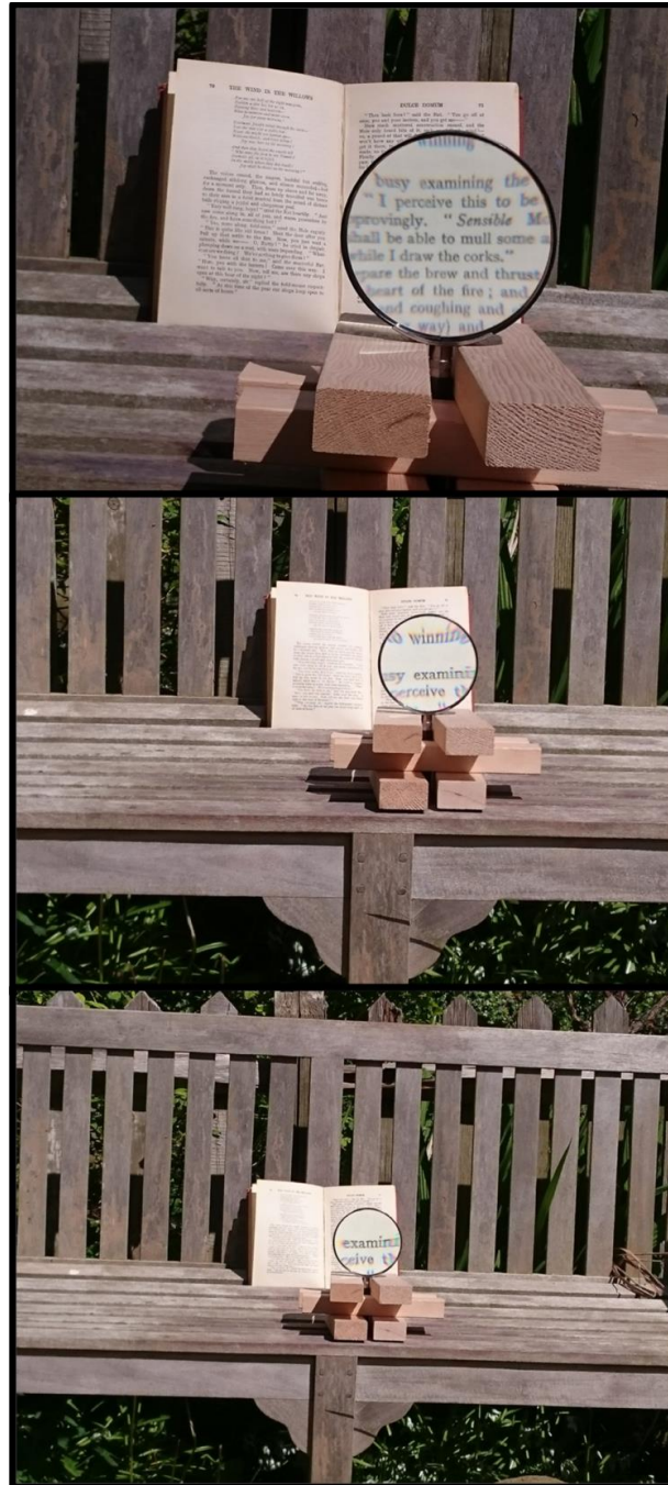
Figure 5. A single convex lens placed in front of text by its own focal length, viewed at distances of 1, 2, and 3 m, respectively.
