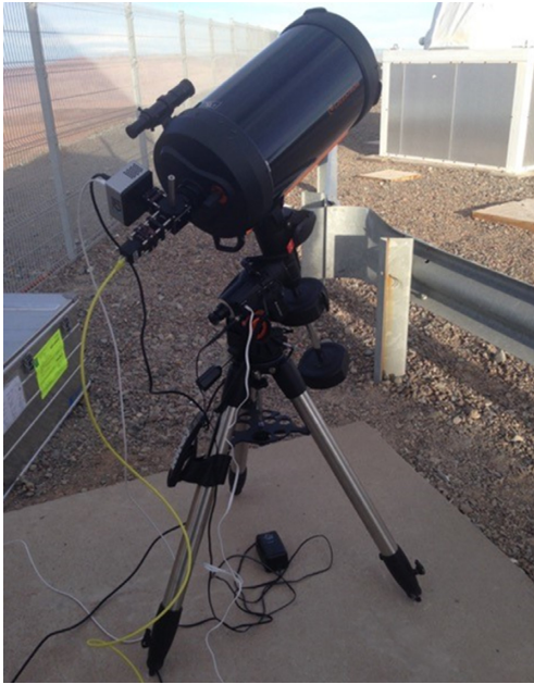
Figure C1. Prototype of the FASS–SHIMM instrument with the optics mounted on a 9 arcsec- F/10 Celestron telescope at the VLT site, Paranal, 2018 (Perera 2018).
