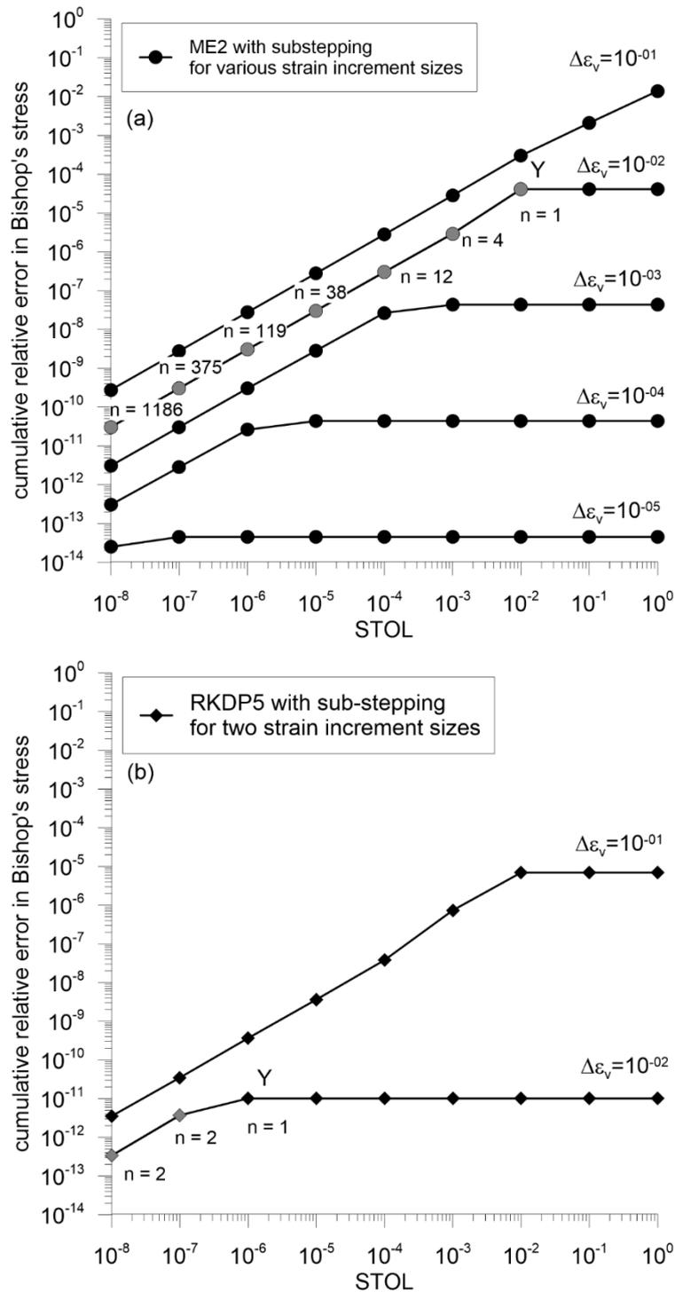
1031 Figure 11. Cumulative relative error behaviour against *STOL* for an elasto-plastic
