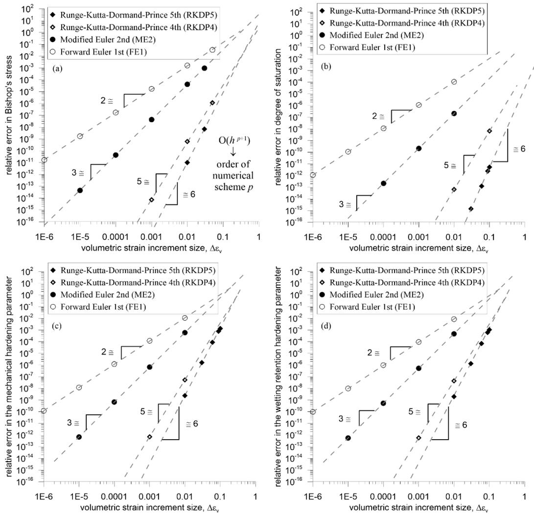
897 Figure 7. Relative error for single-step explicit integration schemes against volumetric
