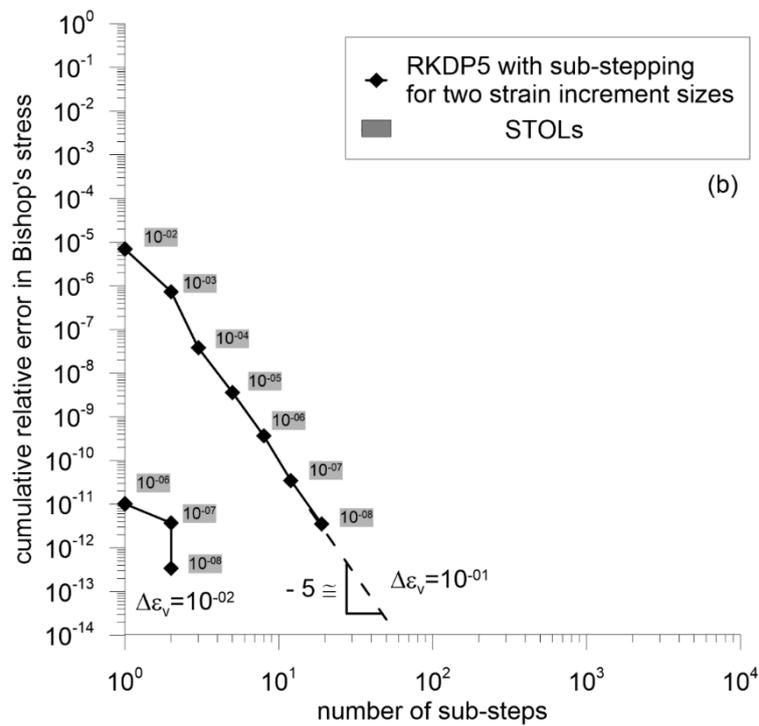
1034 Figure 12. Cumulative relative error behaviour against number of substeps for an elasto-
