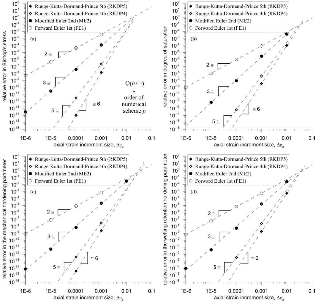
901 Figure 8. Relative error for single-step explicit integration schemes against axial strain
