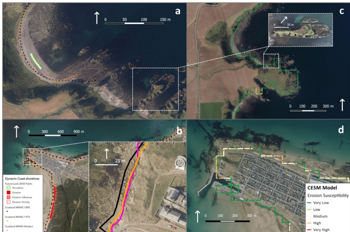
Figure 5. Coastal erosion models for early medieval study sites ((a)—Dynamic Coast shorelines for Dunnicaer and proximity; (b)—Dynamic Coast shorelines for Burghead and proximity (inset showing shorelines on NW face); (c)—CESM data for Dunnicaer and proximity (inset showing aerial view of site and extent of erosion); (d)—CESM data for Burghead).
