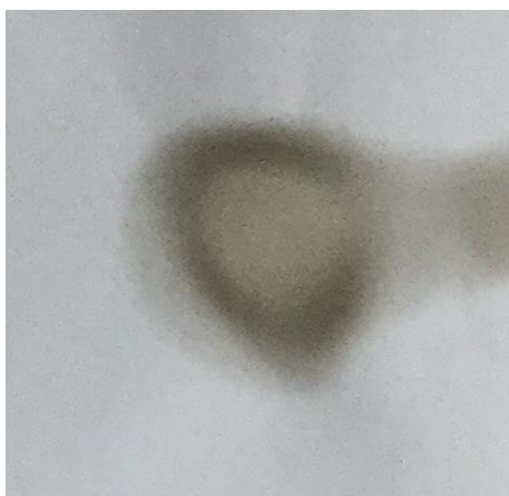
Figure 3. A charred ring formed on a piece of paper held briefly in a candle flame.
