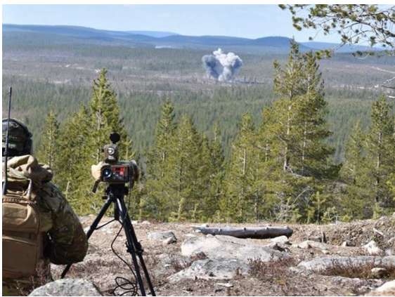
Figure 77. Leonardo's modern Type 163 laser designator during a live fire test. (Picture courtesy of Leonardo.)
