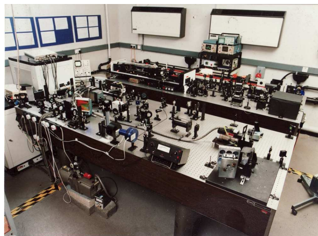
Figure 7. The UK's first table-top terawatt ( T^3 ) system, a 1 J, 1 ps T^3 laser developed at Imperial College by the Laser Consortium, circa 1998. This was the first operational T^3 CPA laser system in Europe, built by PhD student Mary Falden and then Postdoc Roland Smith. (Picture courtesy of Imperial College London.)
