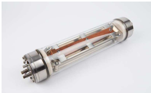
Figure 86. Early Lambertson and Pearson trigger wire pre-ionized TEA laser providing 2.0 J pulse outputs at 1.0 Hz repetition rates from an active laser volume of 100 cm 3 .
