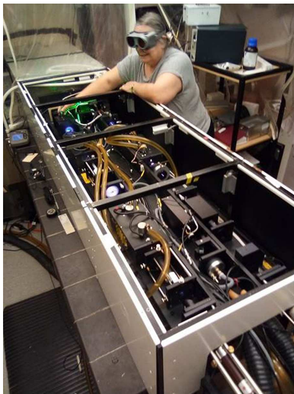
Figure 50. Janet Hull, JEH Lasers, maintaining a JK Lasers Nd:YAG mode locked dye system in 2020 at the Space Geodesy Group, Herstmonceux, East Sussex. Parts of the laser date back to the late 1970s, it was heavily modified in the early 1980s and is still operational.
