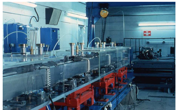
Figure 21. The UK-FEL undulator at Kelvin Laboratory, East Kilbride circa 1983.
