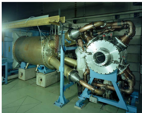
Figure 30. Dave Wood shown with the Sprite e-beam pumped amplifier cell in 1982. (Picture courtesy of STFC.)
