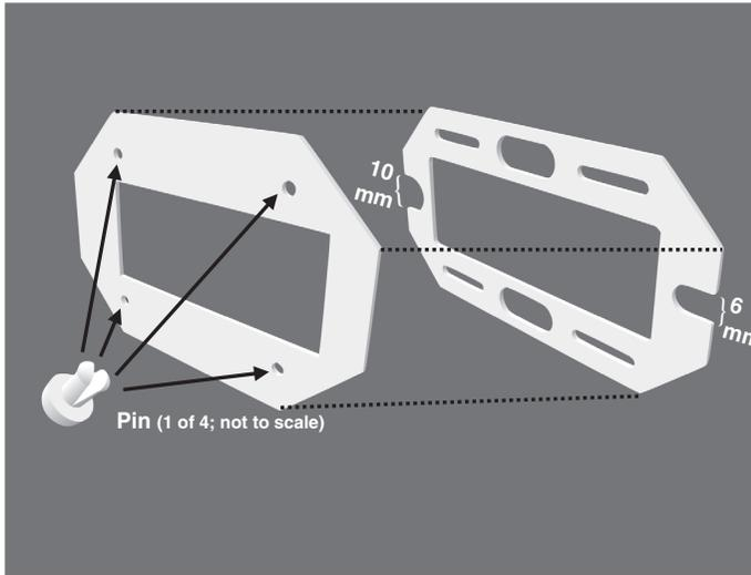
Fig. 1. Schematic of the 3D-printed muscle meter. This version is double-sided with both a 6-mm gap (for small songbirds) and a 10-mm gap (for medium-sized songbirds).
