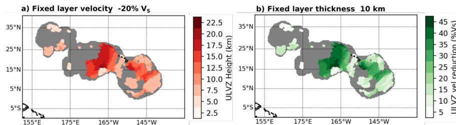
Figure 8: a) Predicted ULVZ heights based on pre/post-cursor arrivals imaged in CBP stacks assuming a layer of constant velocity contrast of -20%. b) Predicted ULVZ velocity contrasts assuming a layer of constant height of 10km.
