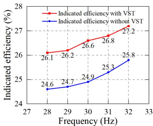
**Fig. 22** Comparison of indicated efficiency
