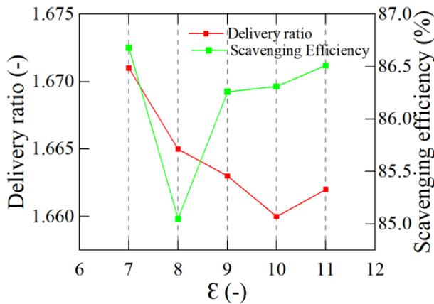
Fig. 12 Delivery ratio and scavenging ratio with different compression ratios
