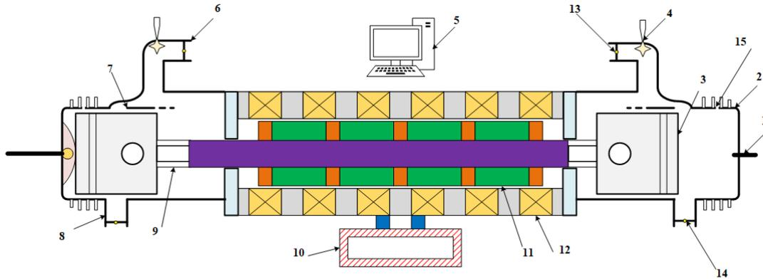
1. Spark plug 2. Cylinder 3. Piston 4. Fuel injector 5. Control system 6. Air-intake tube 7. Scavenging port 8. Exhaust port
