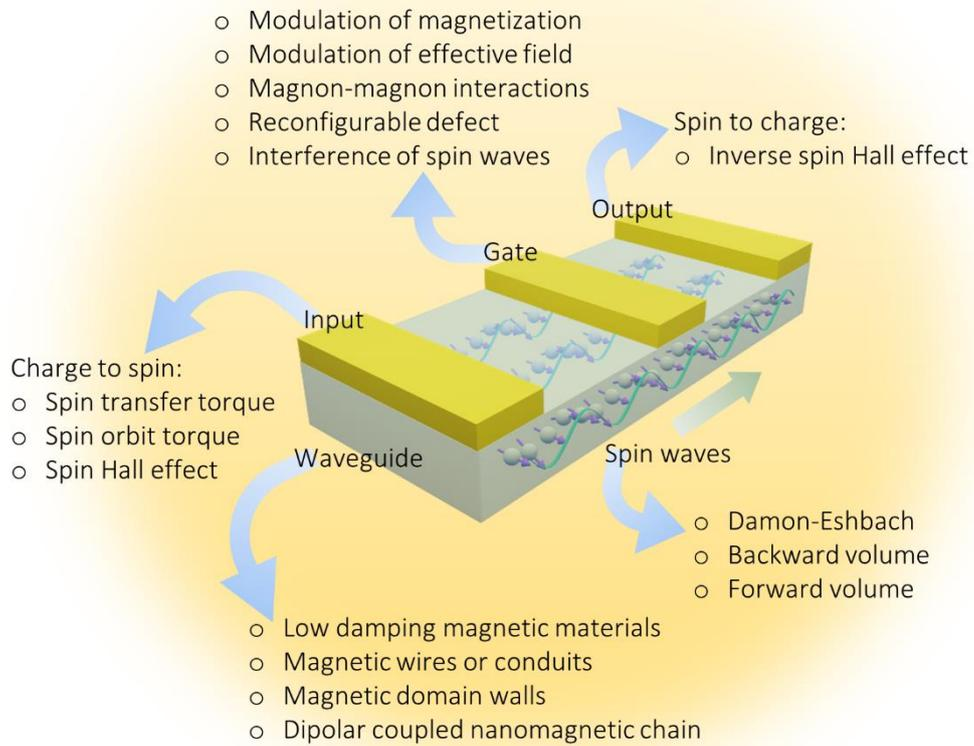
**FIGURE 1:** Schematic of a magnonic device and its building blocks which are associated with a range of phenomena.
