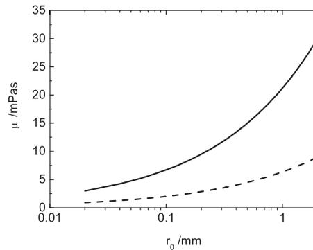
FIG. 12. Lower (dashed line) and upper (solid line) limit of viscosity of fluid for OD measurements for a surface tension of  $45 \text{ mN m}^{-1}$  and density of  $1 \times 10^3 \text{ kg m}^{-3}$  as a function of drop radius,  $r_0$ .
