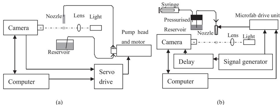
FIG. 1. Schematic of the experimental arrangement for liquid dispensing and drop visualisation of (a)  $\mu\text{l}$  drop and (b) pl droplet.
