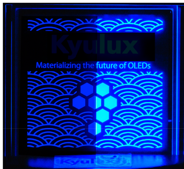
Figure 6. Demonstration of blue hyperfluorescence OLED compared to the sensitizing host on its own. Courtesy of Kyulux Inc.
