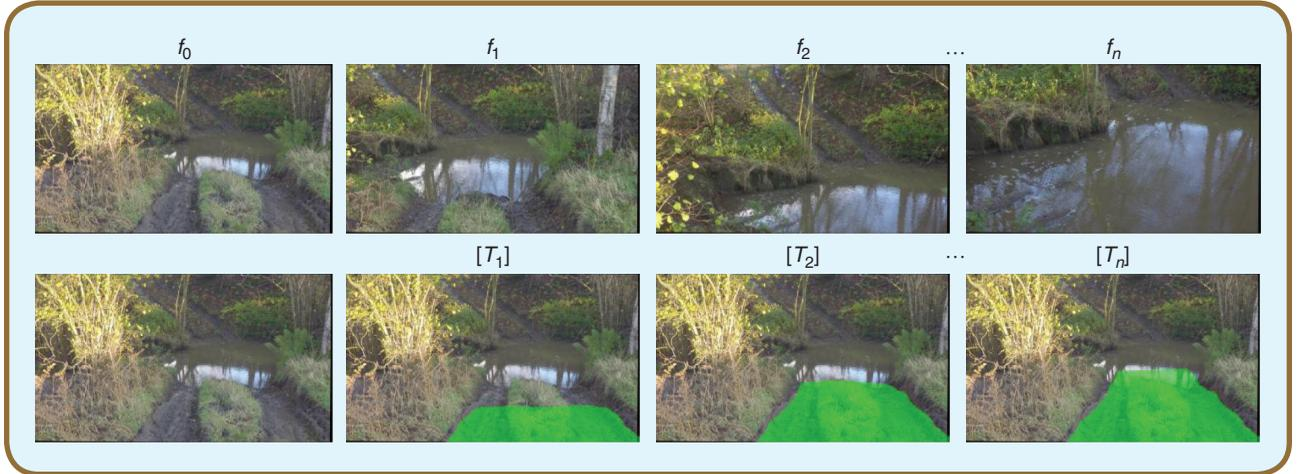
**FIG 1** Example sequence from our data set: starting from frame  $f_0$ , transformation matrices  $[T_1]$  to  $[T_n]$  are computed for camera position in  $n$  subsequent frames, from which vehicle footprint can be calculated and translated back into image space so that path pixels can be labelled. Top row contains original frames  $f_0$  to  $f_n$ , while bottom row shows aggregate computed footprint at each frame overlaid onto  $f_0$ .
