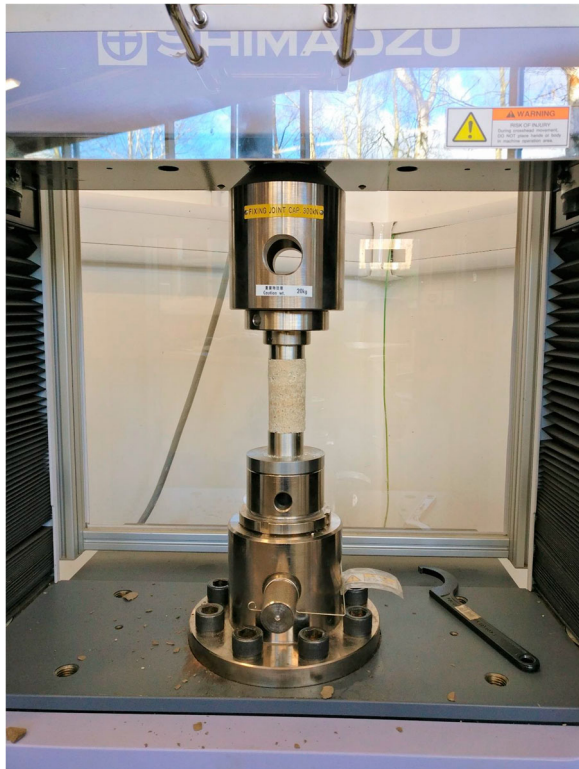
Figure 1. Unconfined compression test setup.
