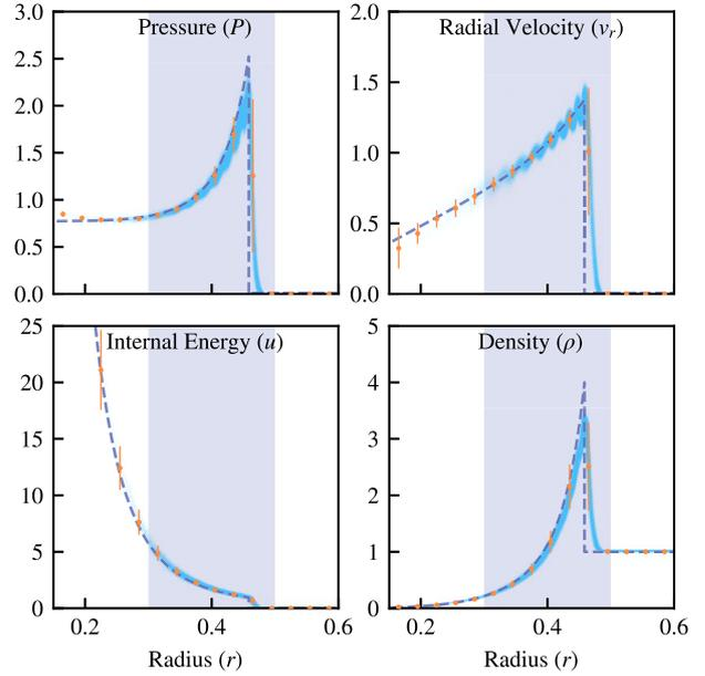
**Figure 5.** Particle properties at  $t = 0.1$  shown against the analytic solution (purple dashed line) for the Sedov–Taylor blastwave. A random sub-set of 1/5th of the particles are shown in blue, with the orange points showing the mean value within equally spaced horizontal bins with one standard deviation of scatter. The background purple band shows the region considered for measuring convergence in Fig. 6. This figure shows the results for a  $128^3$  particle glass file.
