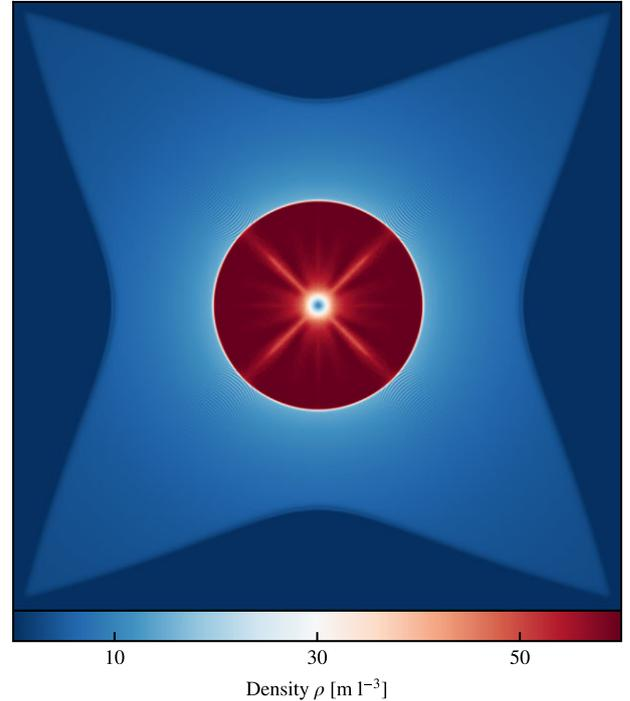
**Figure 10.** A density slice through the centre of the Noh problem at  $t = 0.6$  corresponding to the particle distribution shown in Fig. 9. The SPHENIX scheme yields almost perfect spherical symmetry for the shock, but does not capture the expected high density in the central region, likely due to lower than required artificial conductivity (see Appendix E for more information).
