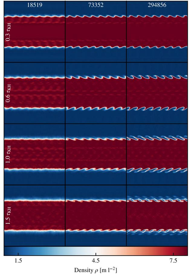
**Figure 14.** The same as Fig. 13, but this time using initial conditions with a significantly higher (1:8 instead of 1:2) density contrast. The initial instabilities are captured well at all resolution levels, but at the lowest level they are rapidly mixed by the artificial conduction scheme due to the lack of resolution elements in the low-density region.
