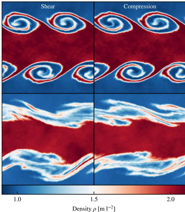
**Figure B3.** Kelvin-Helmholtz test with a density contrast of  $\rho_c = 2$  as in Fig. 13, shown at  $t = 2\tau_{\text{KH}}$  (top) and  $t = 4\tau_{\text{KH}}$  (bottom). We show on the left the simulation with the shear-based conduction speed, and again the compression-based speed on the right. No significant qualitative differences are seen between the two models.
