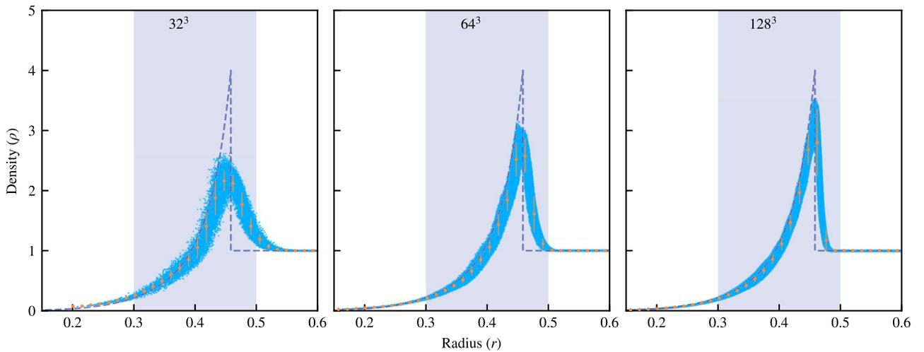
**Figure D1.** The density profile of the Sedov blasts initially presented in Fig. 6. The blue points show the positions of every particle in the volume, the purple dashed line the analytical prediction, and the orange points binned means with error bars showing one standard deviation. The shaded band is the region over which the convergence properties were measured. The text at the top notes the total number of particles in each volume.
