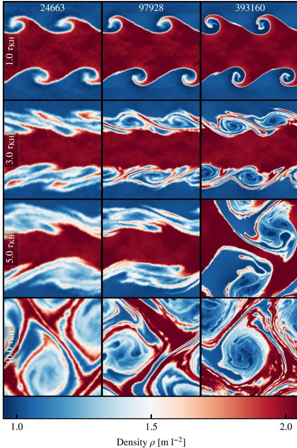
**Figure 13.** Density map of the standard Kelvin–Helmholtz 2D test at various resolutions (different columns, with the number of particles in the volume at the top) and at various times (different rows showing times from  $t = \tau_{\text{KH}}$  to  $t = 10\tau_{\text{KH}}$ ). Despite this being a challenging test for SPH, the instability is captured well at all resolutions, with higher resolution levels capturing finer details.
