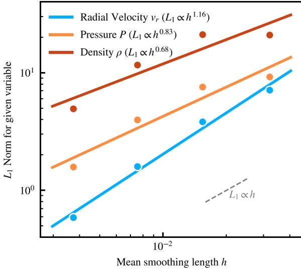
**Figure 11.**  $L_1$  convergence test for various particle properties at  $t = 0.6$  for the Noh problem, corresponding to the particle distribution shown in Fig. 9. The lines without conduction are not shown here as there is a little difference between the with and without conduction case, due to the extremely strong shock present in this test (leading to low values of the viscosity alpha, equation 34).
