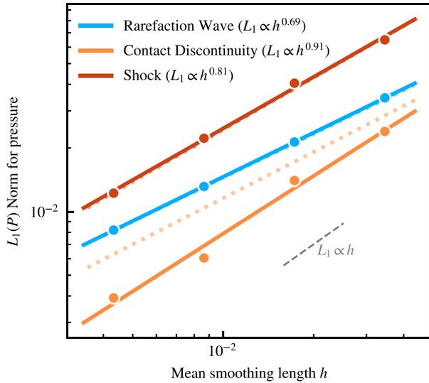
**Figure 4.** Pressure convergence for the three regions in Fig 3. The solid lines show fits to the data at various resolution levels (points) for each region, with the dotted lines showing convergence speed when the artificial conduction term is removed. The dashed grey line shows the expected speed of convergence for shocks in SPH simulations, to guide the eye, with a dependence of  $L_1 \propto h$ .
