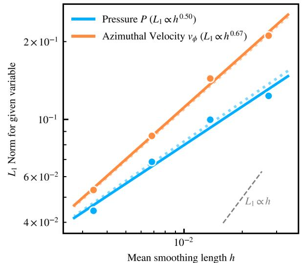
**Figure 8.**  $L_1$  convergence with a mean smoothing length for various particle fields in the Gresho vortex test, measured against the analytic solution within the shaded region of Fig. 7. Each set of points shows a measured value from an individual simulation, with the lines showing a linear fit to the data in logarithmic space. The solid lines show results obtained with the full SPHENIX scheme, with dotted lines showing the results with the artificial conduction scheme disabled.
