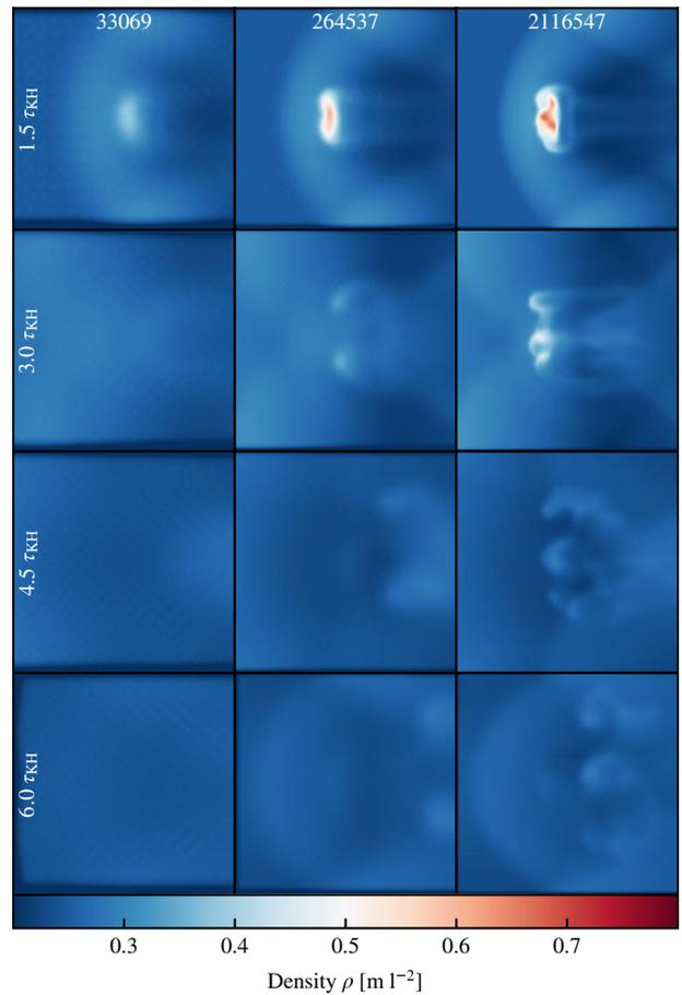
**Figure F2.** A repeat of Fig. 15 but using an SPH-ALE scheme with a diffusive slope limiter. Note, however, that this is one step lower in resolution, due to the additional computational cost required to perform a simulation including a Riemann solver.
