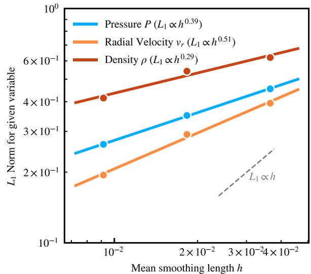
**Figure 6.**  $L_1$  Convergence with mean smoothing length for various particle fields in the Sedov–Taylor blastwave test, measured at  $t = 0.1$  against the analytic solution within the purple band of Fig. 5. Each set of points shows a measured value from an individual simulation, with the lines showing a linear fit to the data in logarithmic space. Dotted lines for the simulation without conduction are not shown as they lie exactly on top of the lines shown here.
