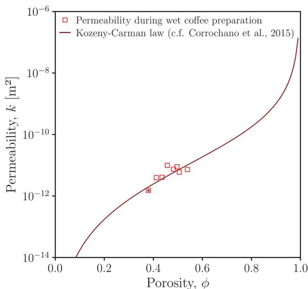
Fig. 7. The fitted permeability  $k$  as a function of porosity  $\phi$  for coffee experiments. The solid curve is a solution to the Kozeny-Carman model with  $C = 180$  using the Sauter coffee grind radius (Eq. (7)) (Ref. 14).
