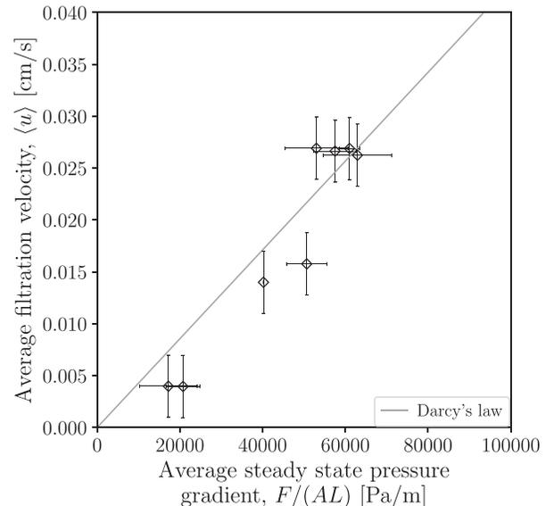
Fig. 6. The filtration velocity  $\langle u \rangle$  as a function of the calculated pressure gradient driving the flow  $F/(AL)$ . The solid curve is the fit to Darcy's law with  $k$  as a free parameter. Here,  $k = (1.34 \pm 0.10) \times 10^{-12} \text{ m}^2$ , where the error is computed from the goodness of fit of Darcy's law to the data.
