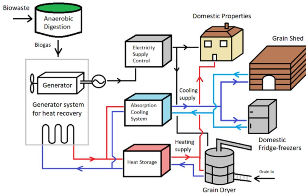
Figure 4 Preliminary trigeneration schematic detailing electricity, heat and cooling flows
