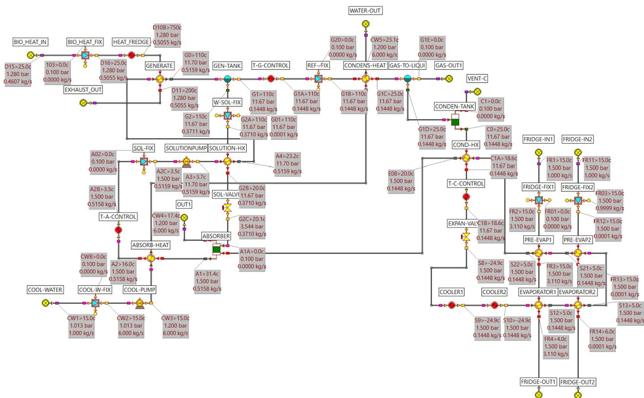
Figure 5 Model Validation: Mass energy balance model for the 17.6 kW Robur absorption chiller
