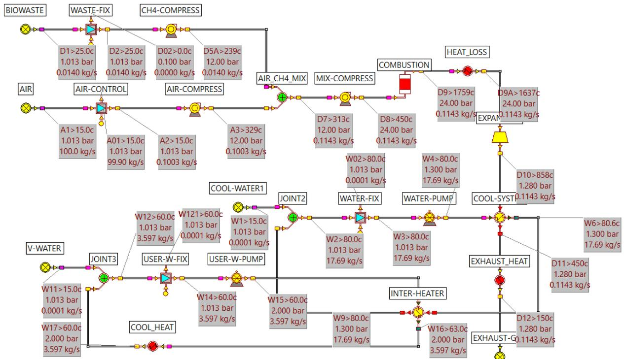
Figure 7 ECLIPSE mass energy balance to model CHP for Option 1
