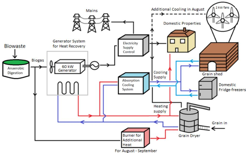
Figure 8 Trigeneration schematic for Options 1 & 2
