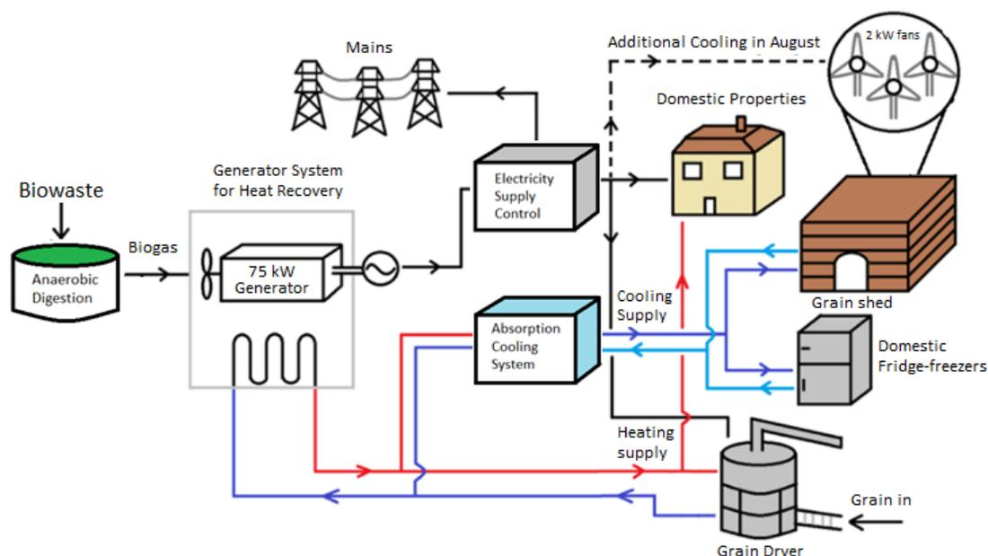
Figure 9 Trigeneration schematic for Option 3
