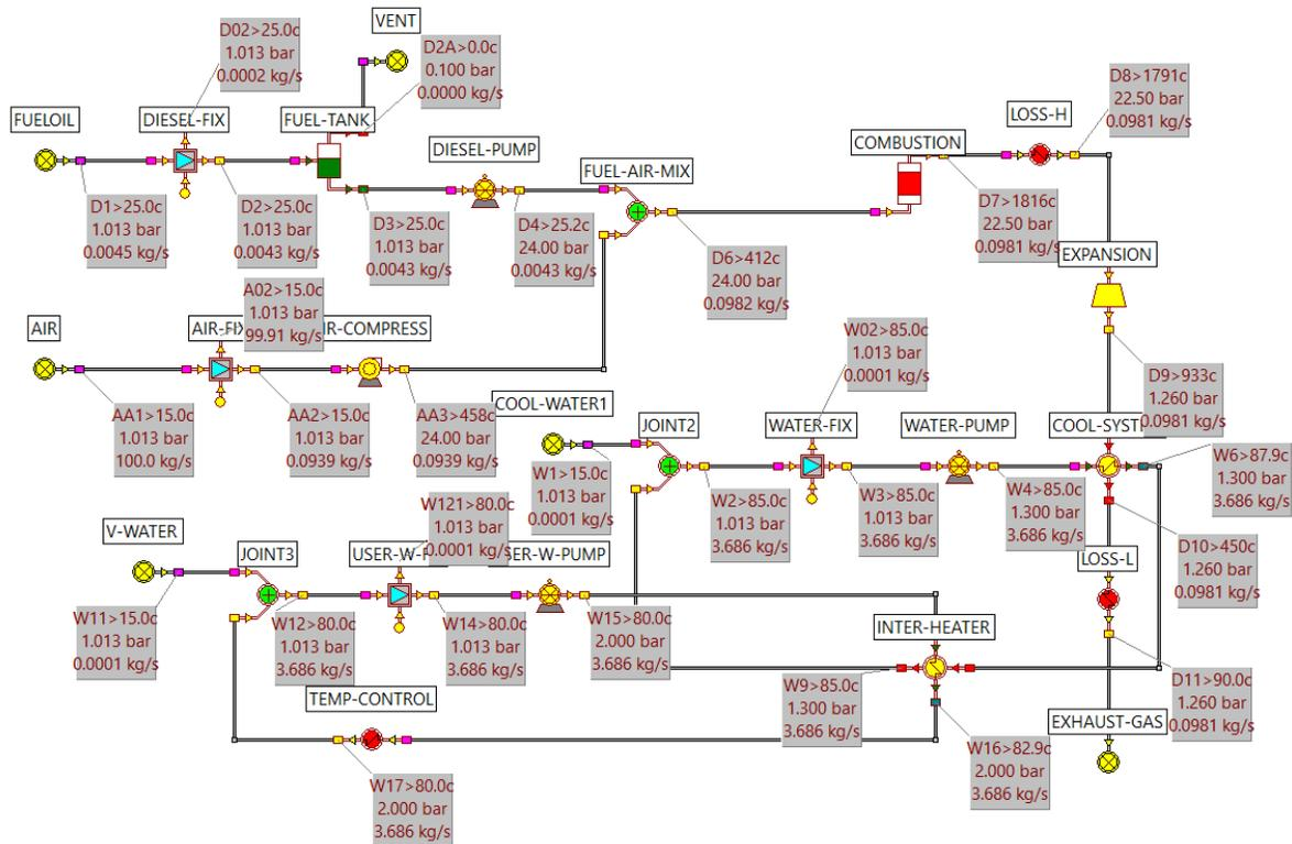
Figure 6 Model Validation: Mass energy balance model for the 60 kW Engine
