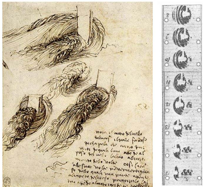
Fig. 1: (Left) Leonardo da Vinci, sketches of the flow around bluff bodies partially immersed in a water stream (1513). (Image mirrored for text reading), (Right) Henri Bénard first cinematography of alternating vortices (Kármán-Bénard wake) past a cylinder towed in water. 13
