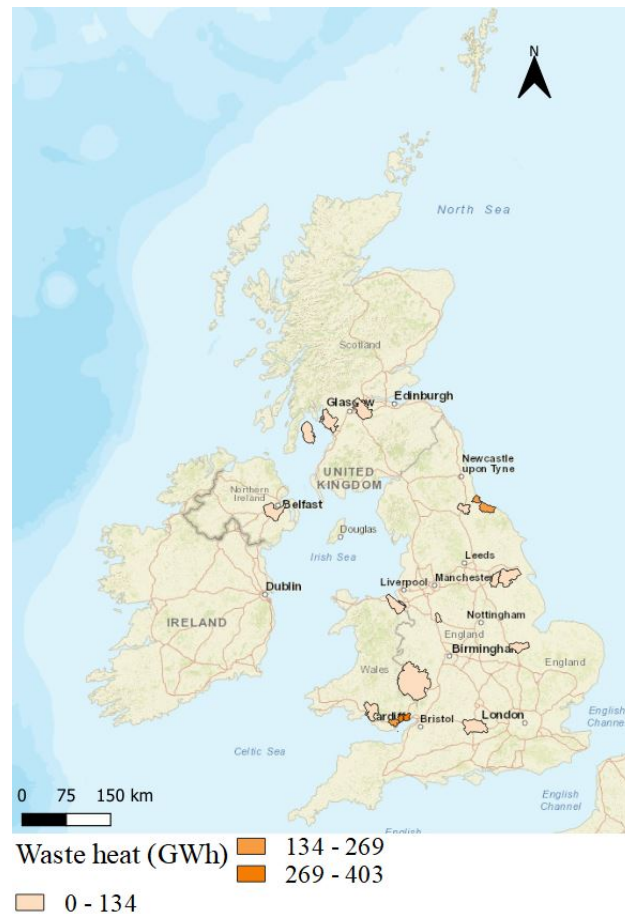
Figure 9: Distribution of estimated waste heat from the UK iron & steel sector by Local Authority area.
