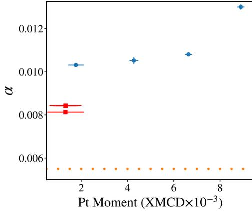
FIG. 5: Damping and XMCD signal as a function of Cu spacer thickness in the CoFe/Cu( $t$ )/Pt. The circles represent the measured damping values at best fitting XMCD values (from 0 to 2 nm) and the square points represent the damping values for higher Cu SL thicknesses. The dotted line represents the damping of the native CoFe.
