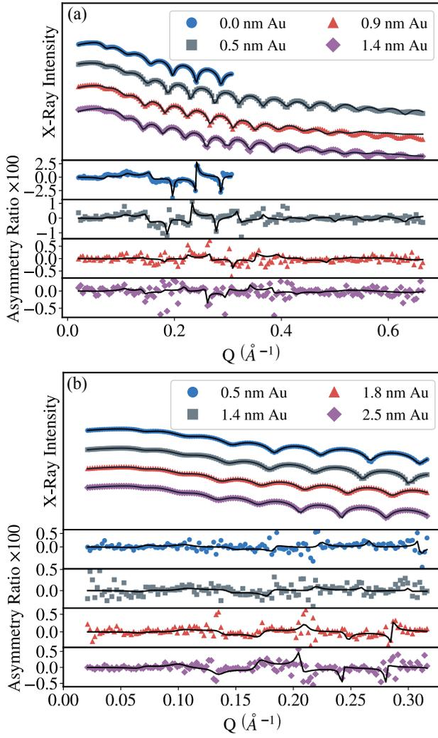
FIG. 9: (a) Measured reflectivity profiles (upper pane) at the Pt  $L_3$  edge with corresponding X-ray helicity asymmetry ratio (lower panes) for four nominal thicknesses of Au spacer layer in a Cu/CoFe/Au/Pt structure. (b) The same measurements at the Au  $L_3$  edge. The asymmetry ratio is as defined in the previous sections. The solid lines represent best fitting models to both the structural and magnetic data.
