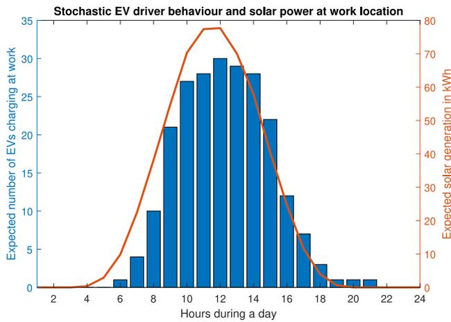
Fig. 3. Stochastic number of EVs and average hourly solar power generation with PV system at the charging station for workplace location.
