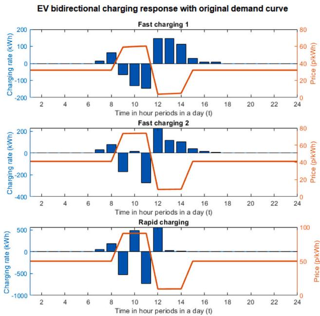
Fig. 6. EV charging profiles as a response to prices with original demand curve using different charging type cases and bidirectional capability.
