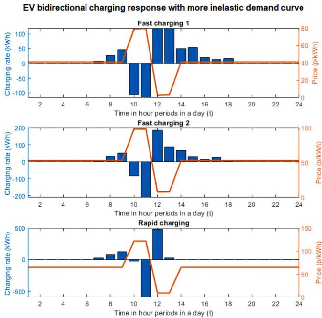
Fig. 9. EV charging profiles as a response to prices with more inelastic demand curve using different charging type cases and bidirectional capability.
