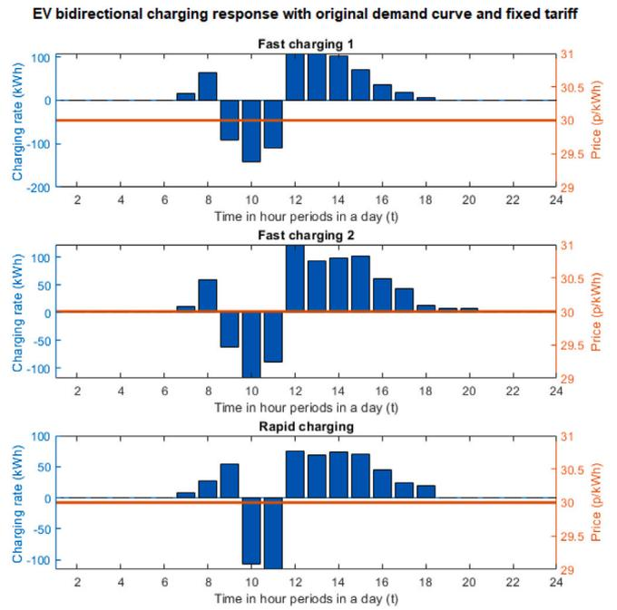
Fig. 10. EV charging profiles as a response to fixed prices with original demand curve using different charging type cases and bidirectional capability.
