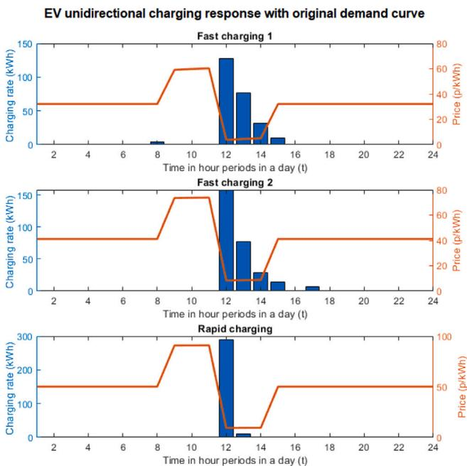
Fig. 7. EV charging profiles as a response to prices with original demand curve using different charging type cases and unidirectional capability.
