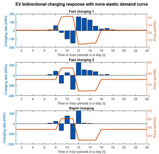
Fig. 8. EV charging profiles as a response to prices with more elastic demand curve using different charging type cases and bidirectional capability.
