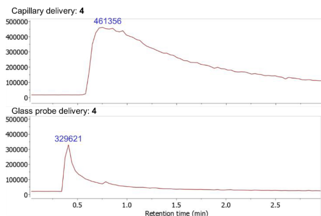
Figure 4. Comparison of total ion count (TIC) signals obtained using ASAP (top) and glass delivery probe ASAP (bottom) MS techniques with a sample of [\text{CoBr}_2(\text{dtbpx})] ( 4 ).
