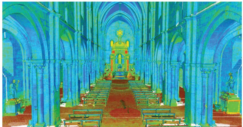
Figure 3. Interior view of the church from point cloud.
