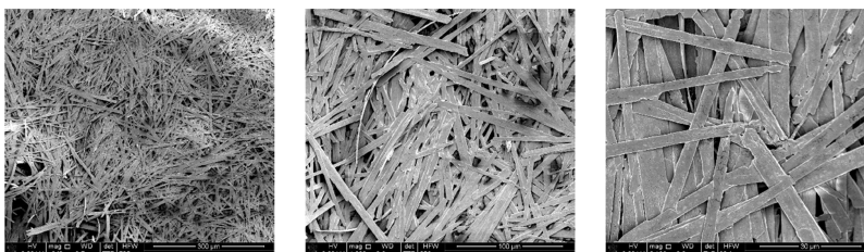
Figure 15. SEM micrographs of the dried xerogel of 1 benzyl alcohol at 5 wt %.
